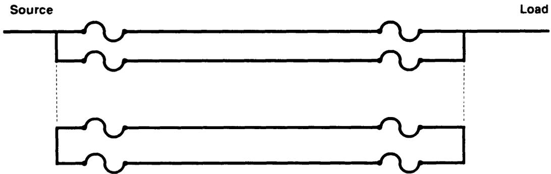
Figure 7. Protection of Parallel Power Wires
