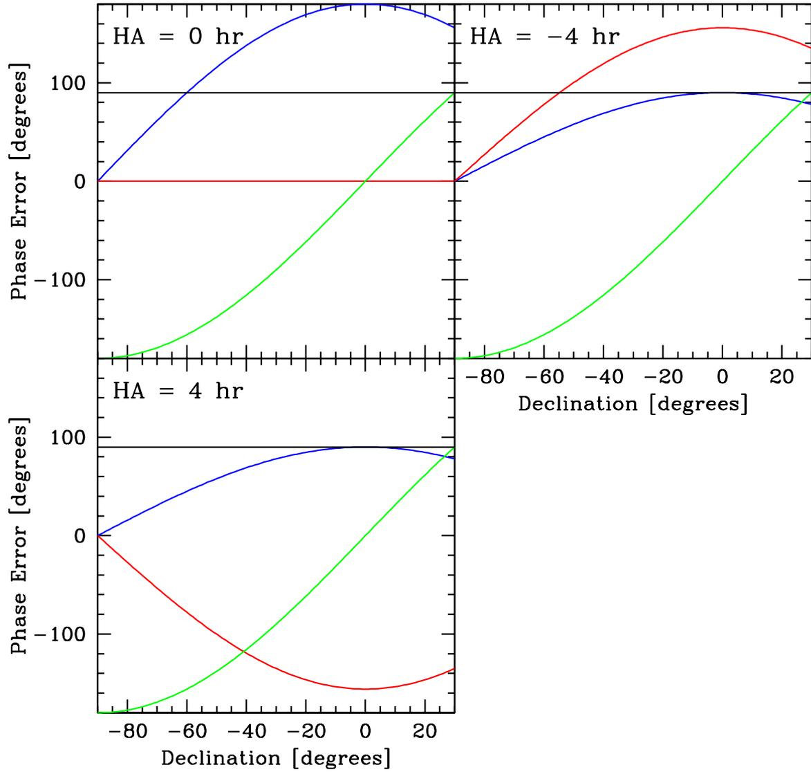
Fig. 2.— Observed Phase Errors versus Declination at Three Hour Angles arising from errors in the adopted baselines, assuming a source at declination of  $-30^\circ$ . Blue:  $\Delta X = 0.5\lambda$ . Red:  $\Delta Y = 0.5\lambda$ . Green:  $\Delta Z = 0.5\lambda$ . Black:  $\phi_{instr} = 0.25\lambda$ .
