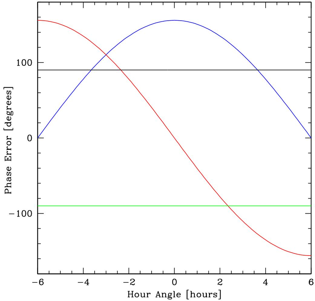
Fig. 1.— Observed Phase Errors versus Hour Angle arising from errors in the adopted baselines, assuming a source at declination of  $-30^\circ$ . Blue:  $\Delta X = 0.5\lambda$ . Red:  $\Delta Y = 0.5\lambda$ . Green:  $\Delta Z = 0.5\lambda$ . Black:  $\phi_{instr} = 0.25\lambda$ .
