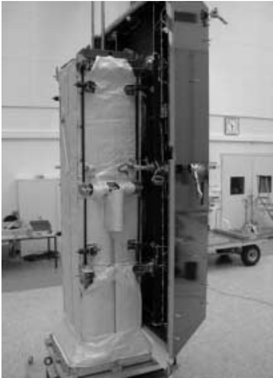
Fig. 4-12: Side-mounted Multiple Satellite Dispenser for Two Spacecraft (Note: only one spacecraft shown in this photo)
