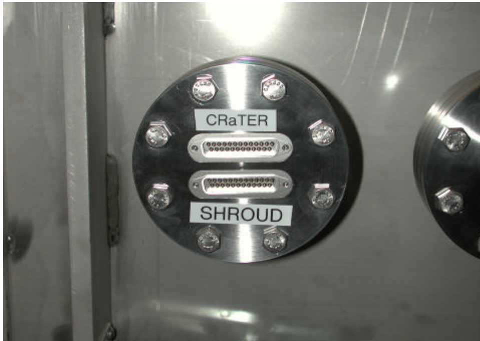
Figure 8. Vacuum Feedthrus for CRaTER and Shroud, 25 pin D-Sub Male
