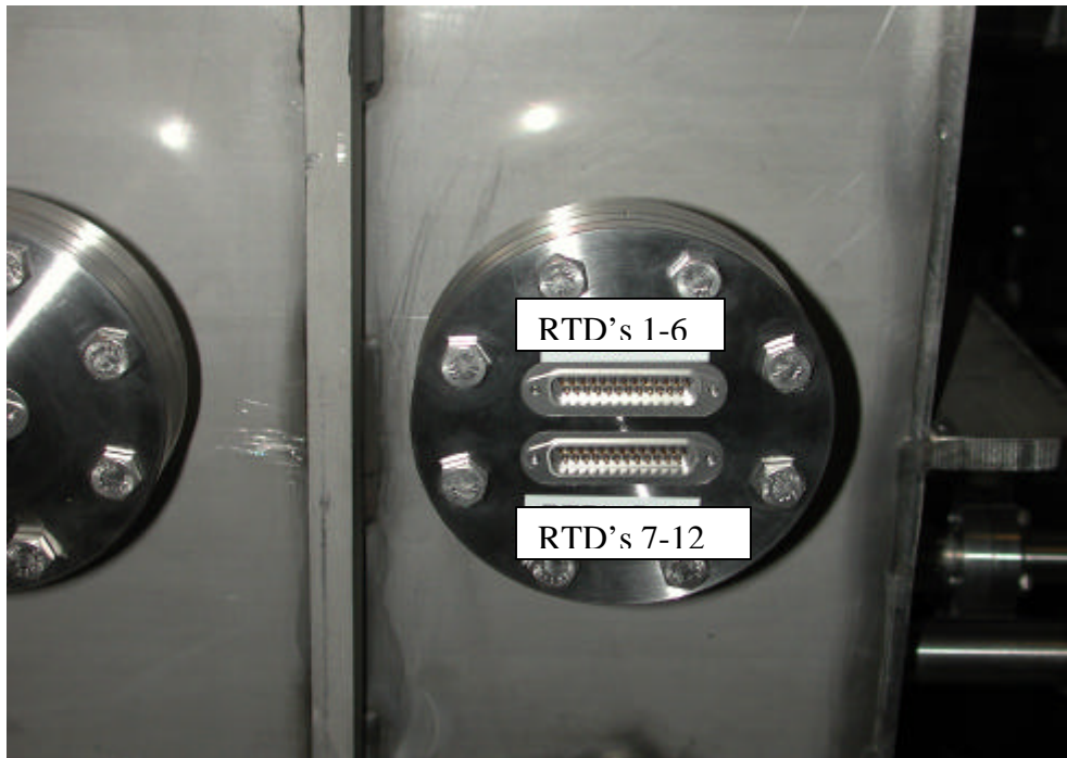
Figure 10. Temperature Monitoring RTDs. 25 pin D-sub, Male.
