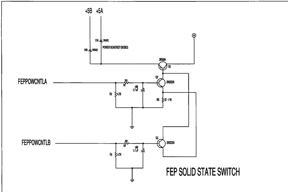
FIGURE 2. Solid State Switch and Control
