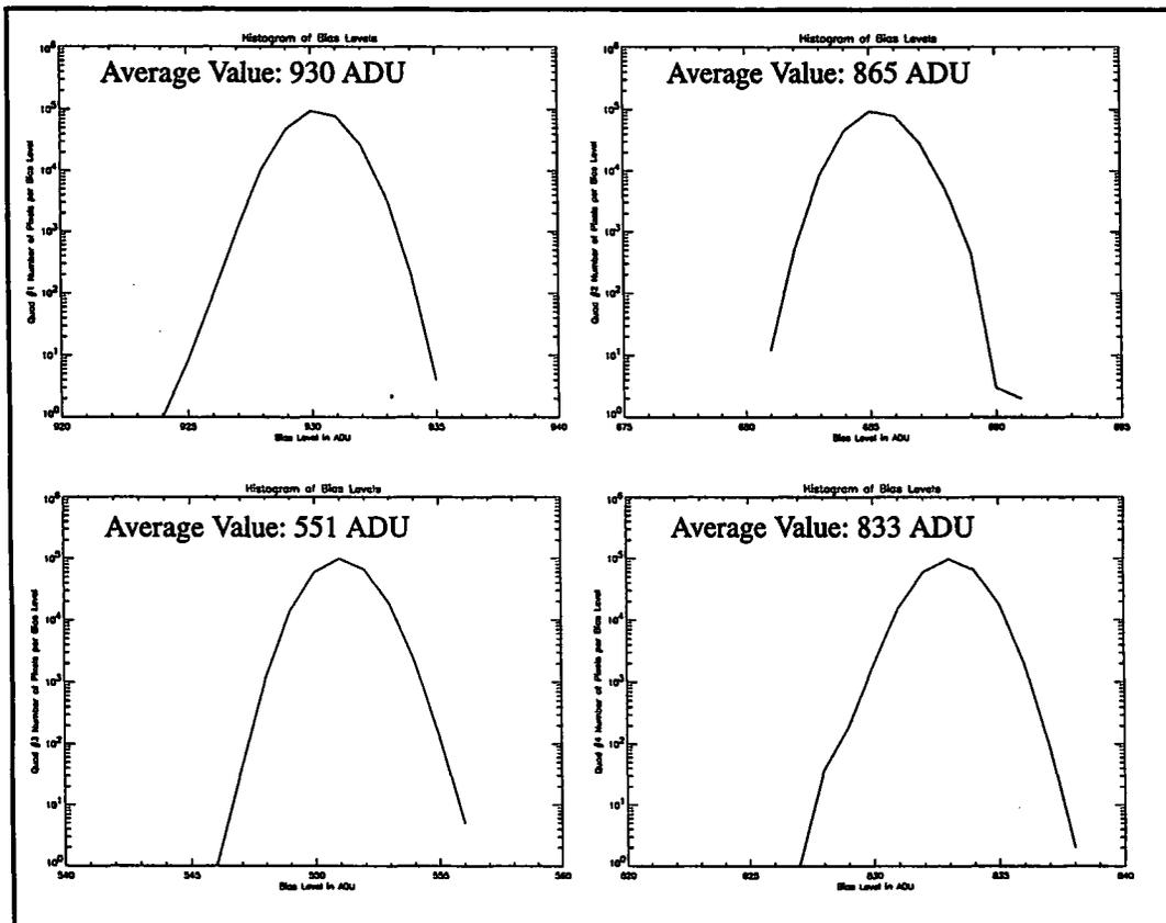
**Figure 2: Histograms of Pixel by Pixel Bias Levels**
