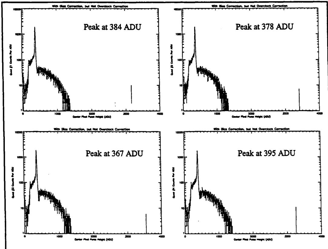
Figure 5: Center Pixel Pulse Heights without Frame Bias Correction
