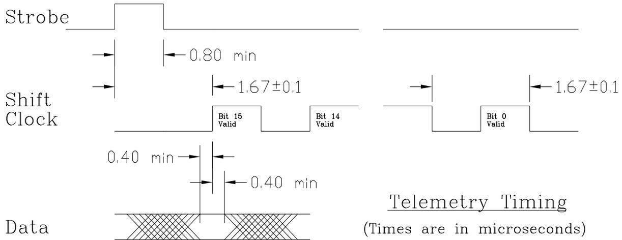
The read strobe tells the FC Instrument to latch the 16-bit telemetry word into a shift register. On the rising edge of each clock pulse the DPU reads the next bit, and on each trailing edge the FC advances the next bit in the register to the output node. A value of +5volts is defined to be a Logical One.
