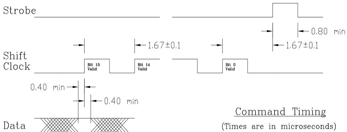
On each rising edge of the shift clock, the FC Instrument reads a data value into a shift register; on the trailing edge of the shift clock the DPU updates the data. After 16 clock pulses a strobe pulse validates completion of the command and is used to latch the full command word into the instrument. A value of +5volts is defined to be a Logical One. Status from FC
