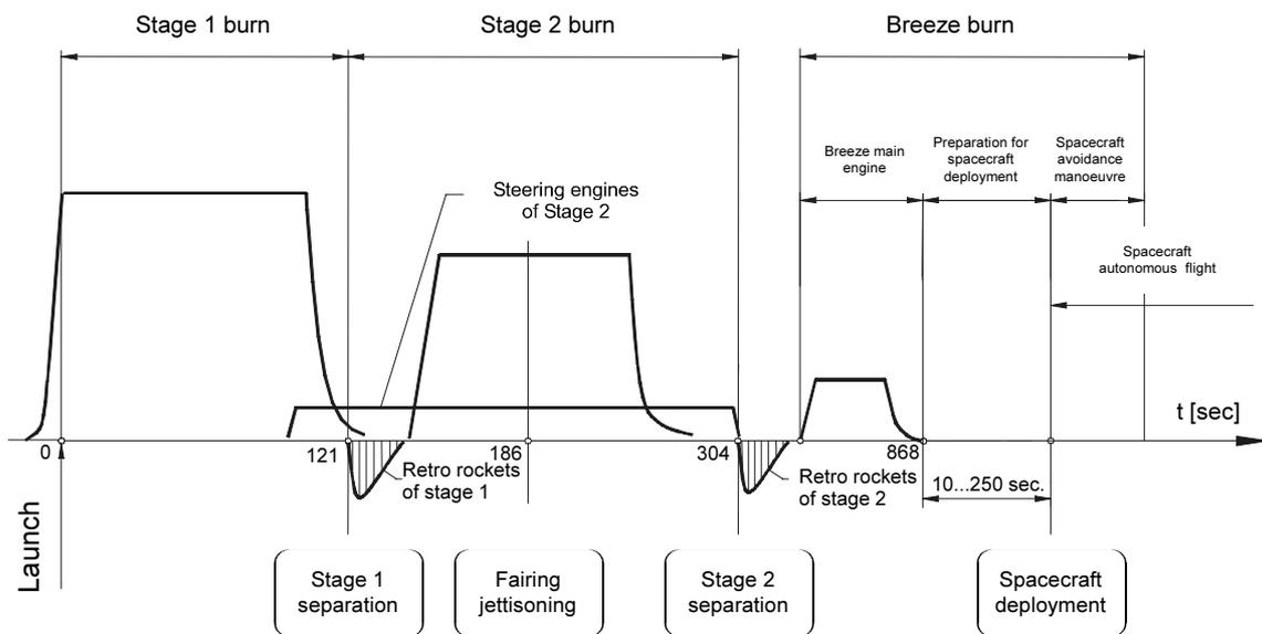
Figure 3-7 : Flight sequence for LEO 300 km
