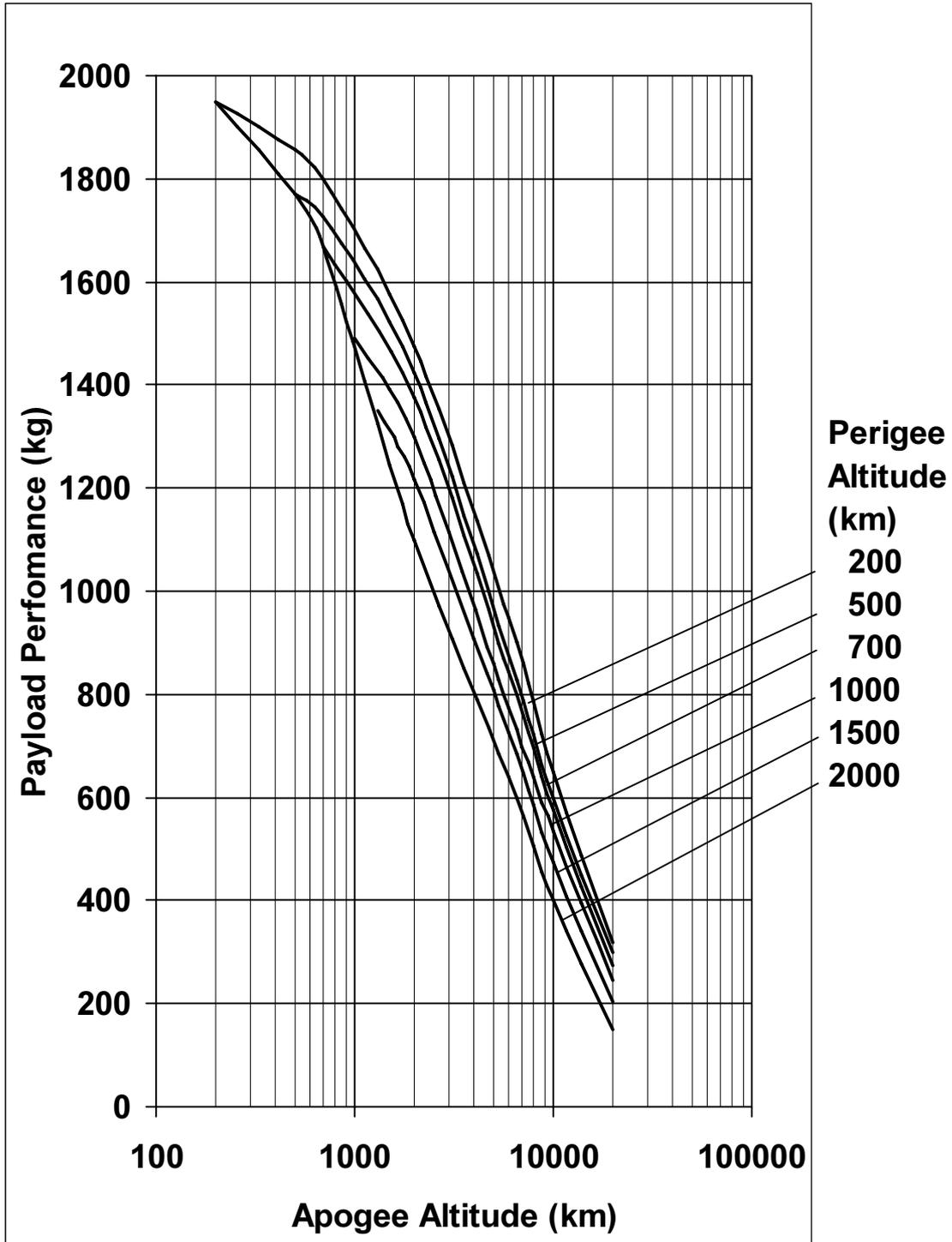
Figure 3-3: Performance for Elliptical Orbits at  $i = 63^\circ$
