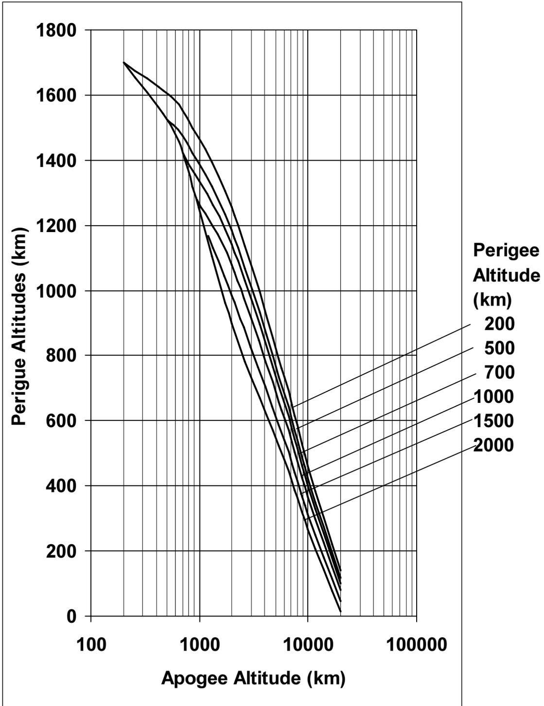
Figure 3-5: Performance for Elliptical Orbits at  $i = 82^\circ$
