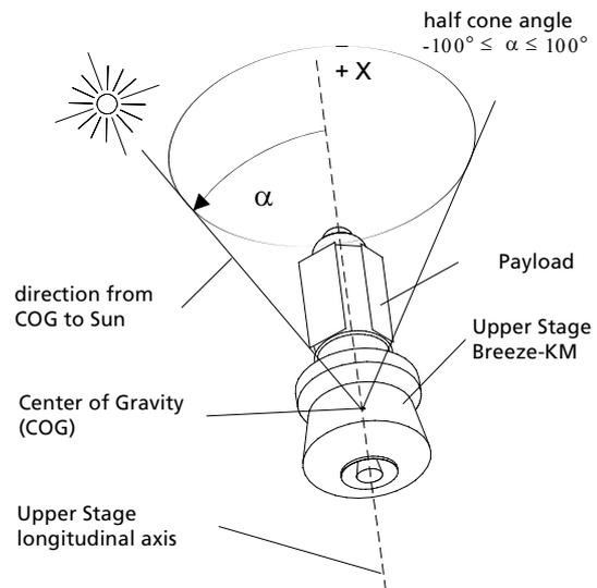
Figure 3-1 (1) : *Breeze-KM* Sun orientation during drift phase
