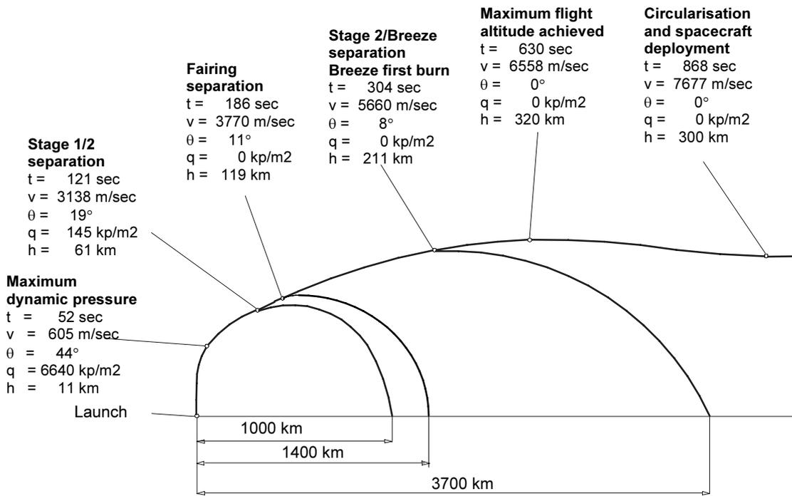
Figure 3-6 Ascent trajectory for LEO 300 km
