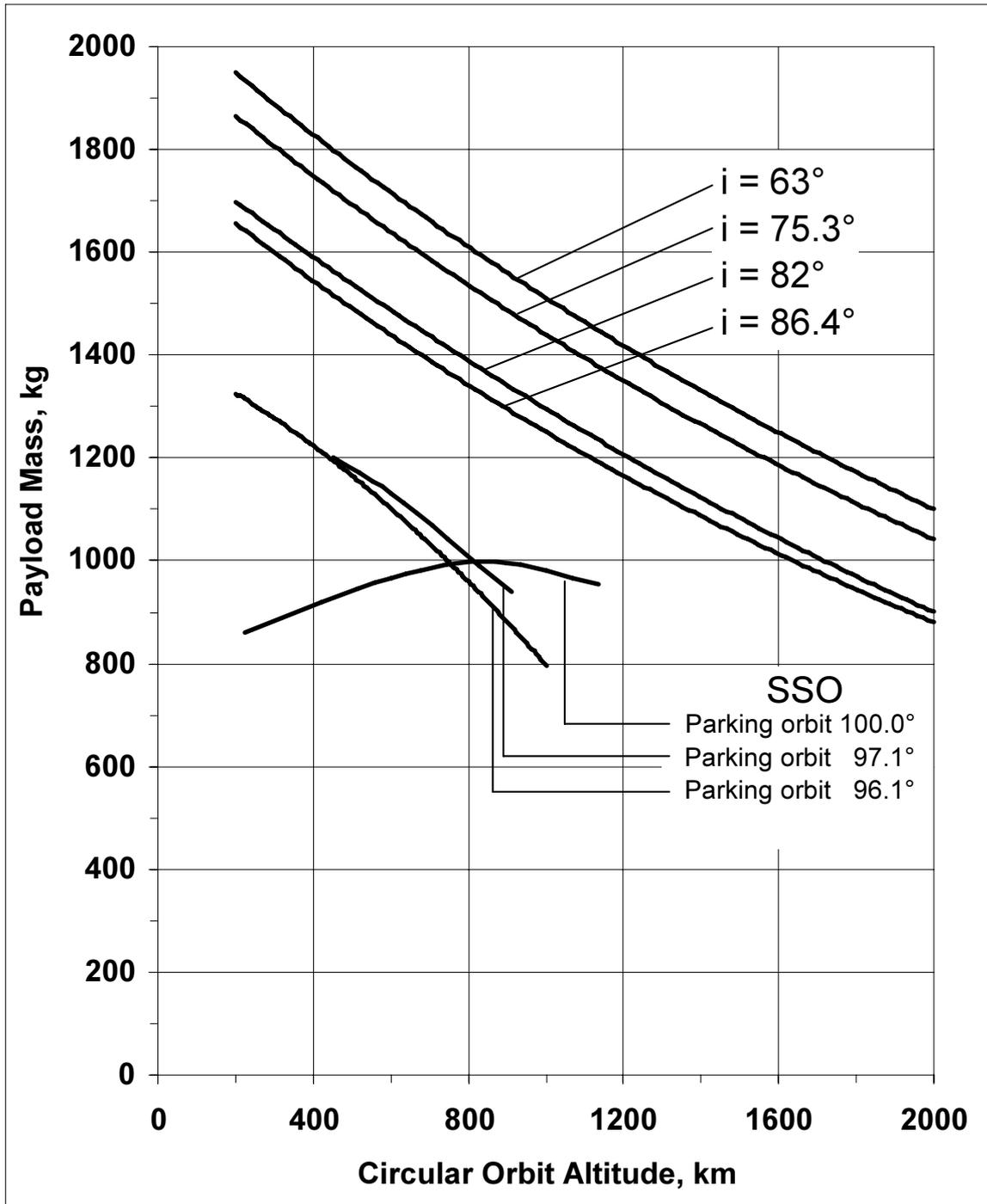
Figure 3-2: Performance Capabilities for Circular Orbits
