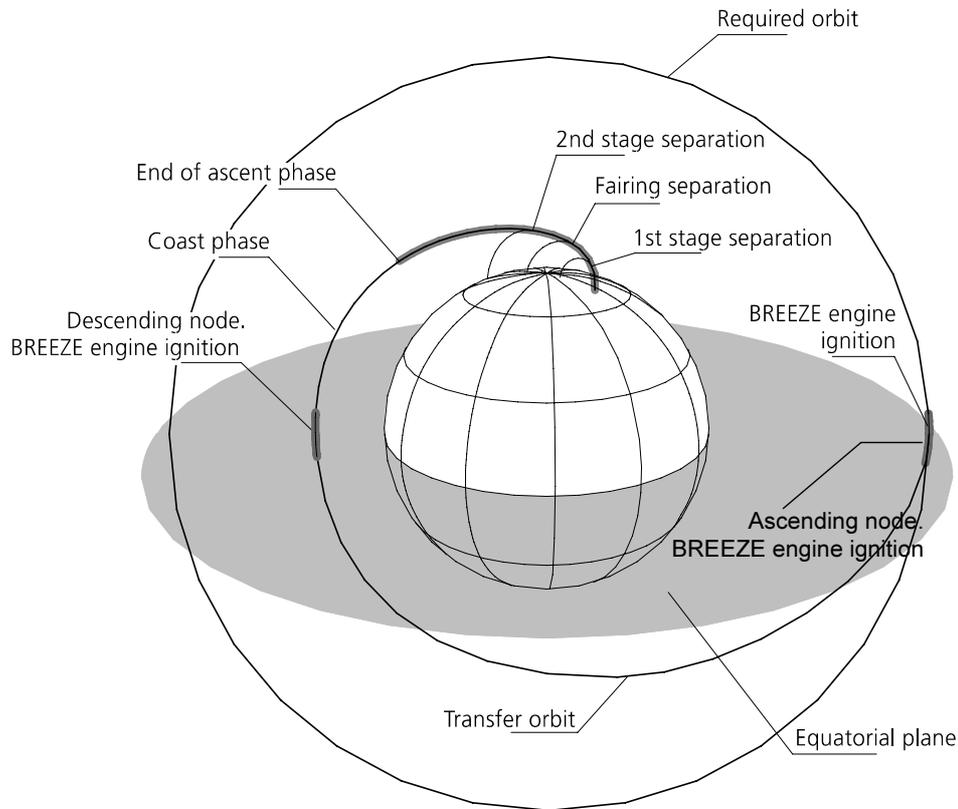
Figure 3-12 : Sun-synchronous Injection Scheme
