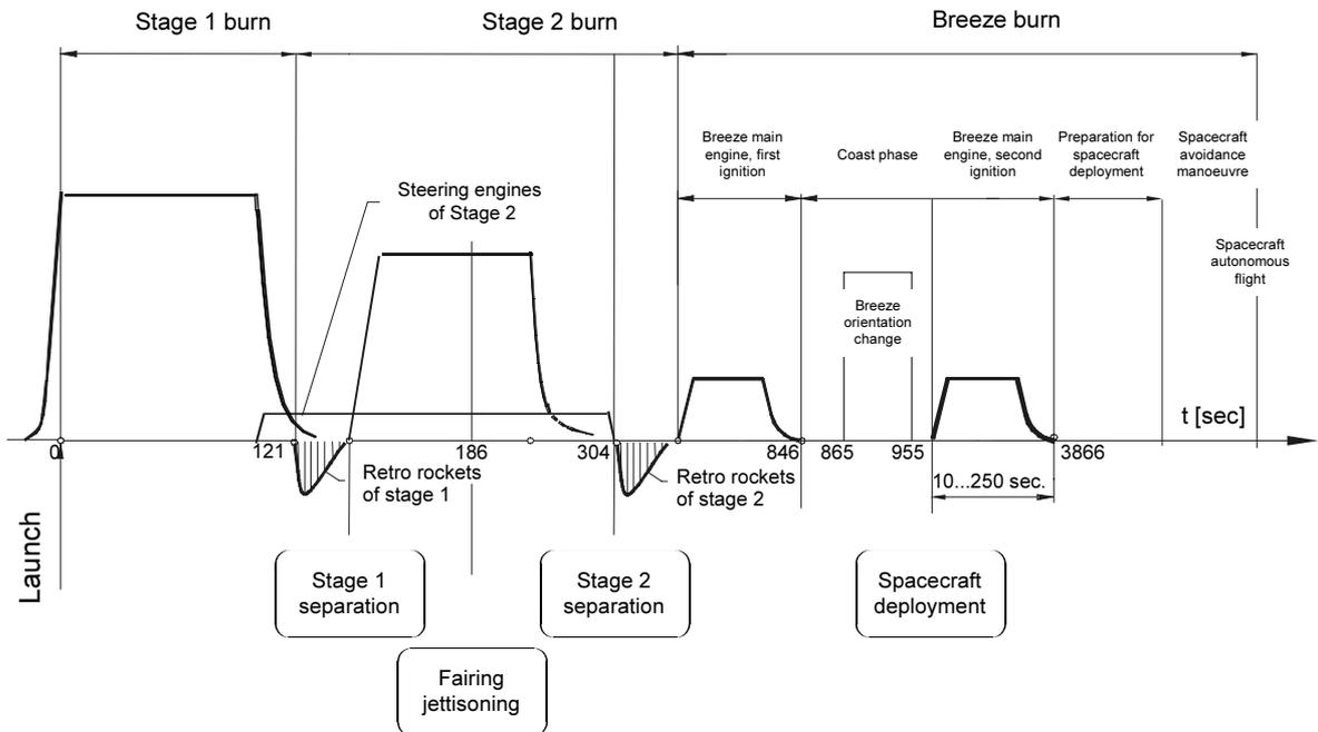
Figure 3-9 : Flight sequence for LEO 700 km
