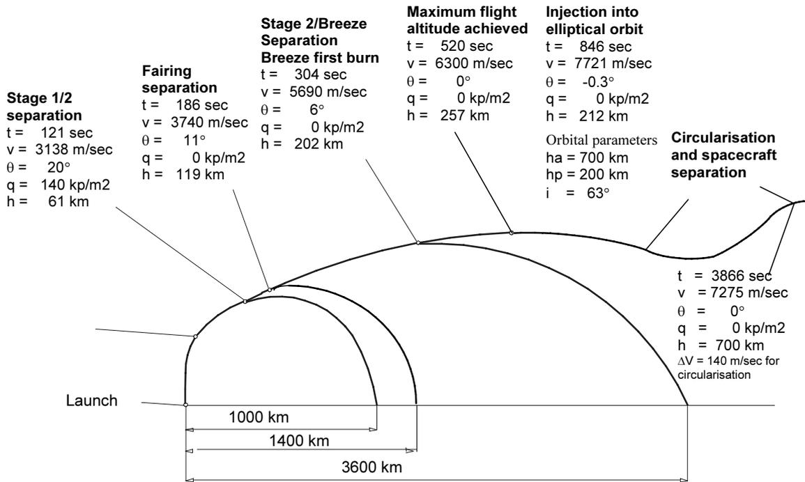
Figure 3-8 : Ascent trajectory for LEO 700 km
