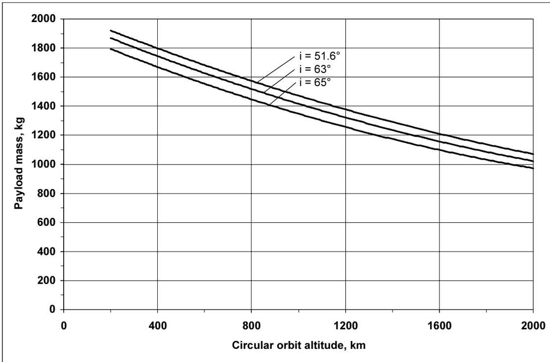
Figure 3-13: Payload Performance for Circular Orbits from Baikonur Cosmodrome
