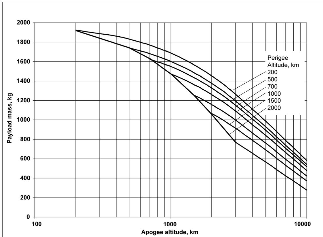
Figure 3-14: Payload Performance for Elliptical Orbits from Baikonur Cosmodrome
