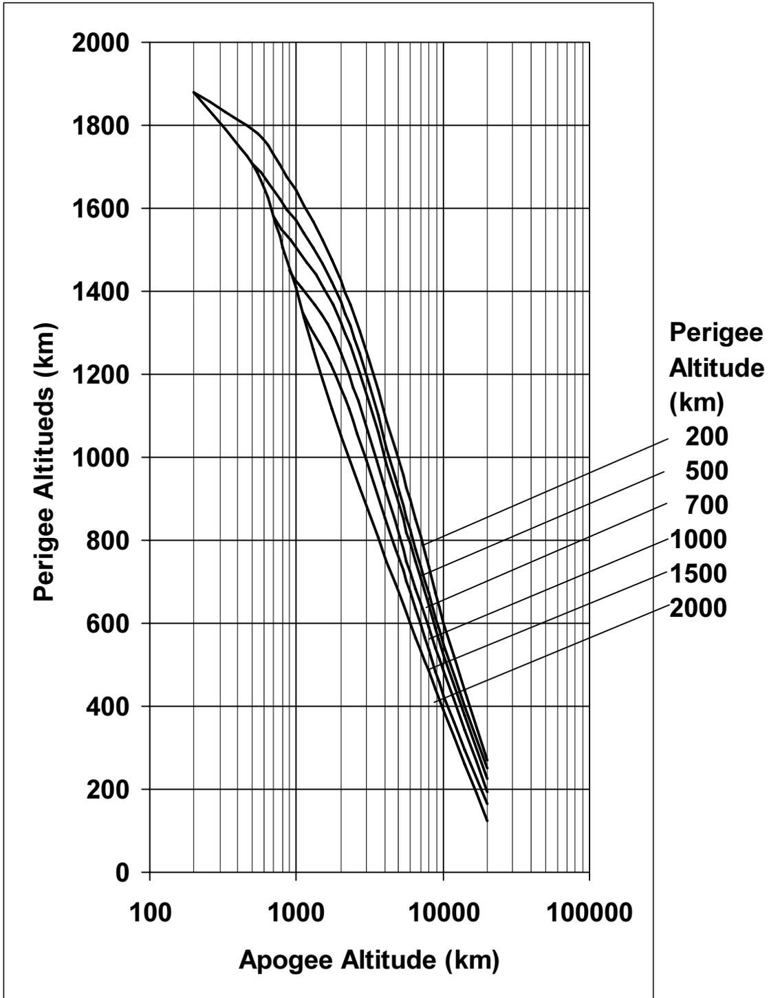
Figure 3-4: Performance for Elliptical Orbits at  $i = 75.3^\circ$
