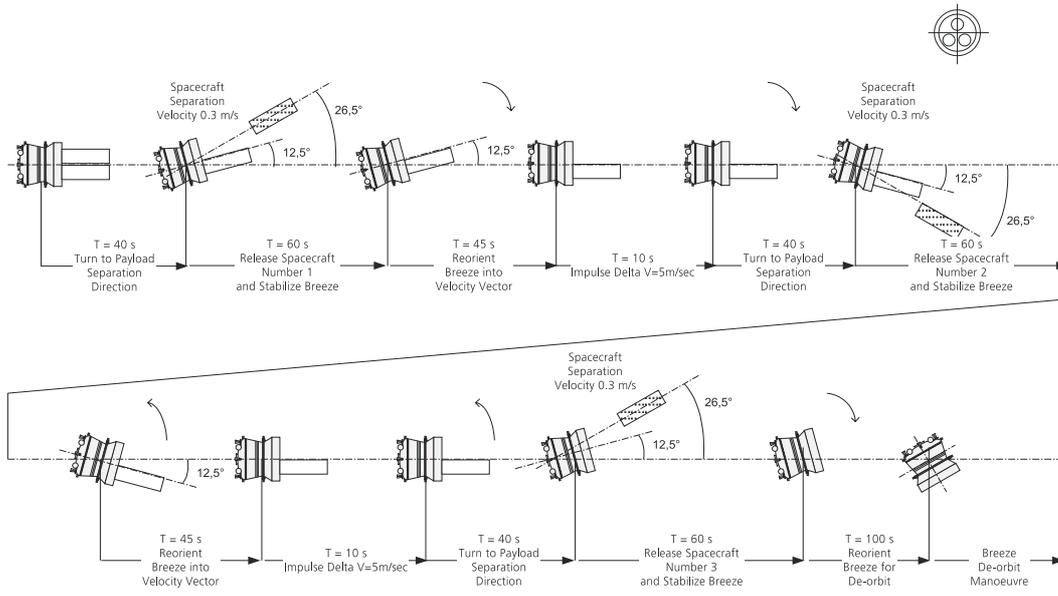
Figure 3-15 : Multiple Payload Deployment Scheme
