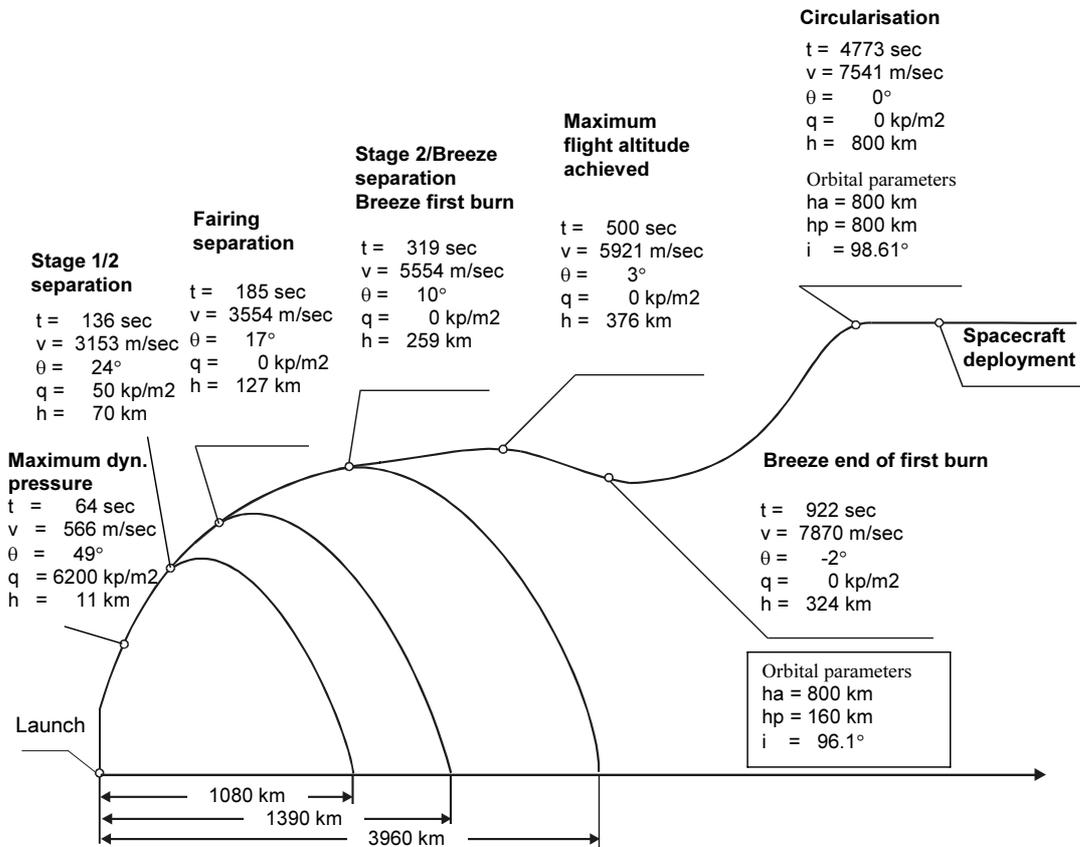
Figure 3-10: Ascent Trajectory for a 800 km/98.6 deg inclined SSO
