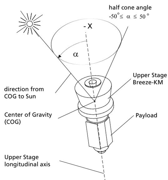
Figure 3-1 (2) : *Breeze-KM* Sun orientation during drift phase
