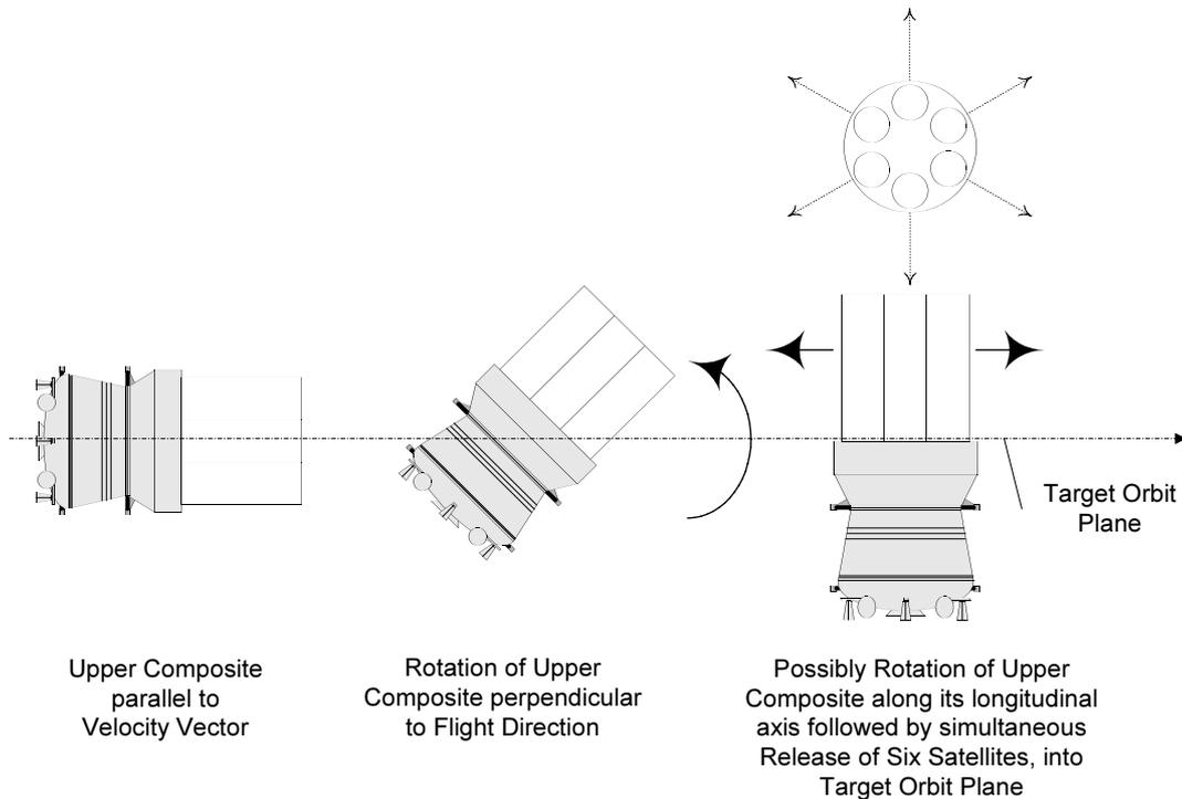
Figure 3-16 : Simultaneous Deployment of Six Spacecraft
