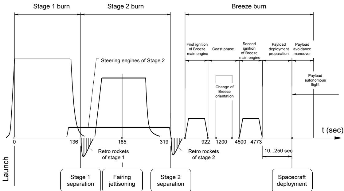
Figure 3-11: Flight Sequence for a 800 km/98.6 deg inclined SSO
