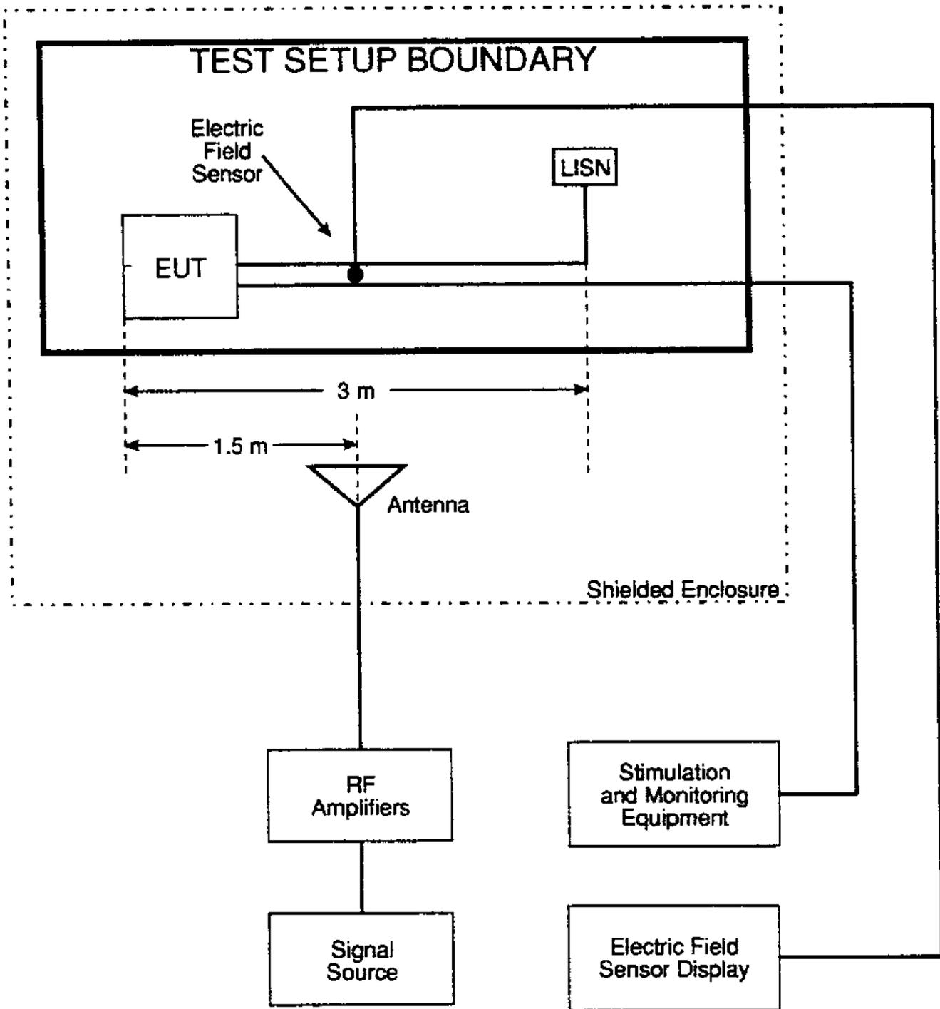
FIGURE RS103-1. Test equipment configuration.
