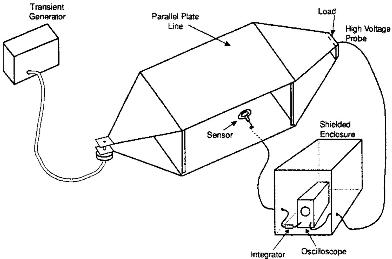
FIGURE RS105-1. Typical calibration setup using parallel plate radiation system.
