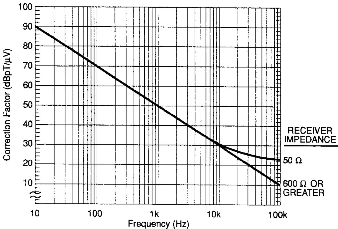
FIGURE RE101-1. Loop sensor correction factor.
