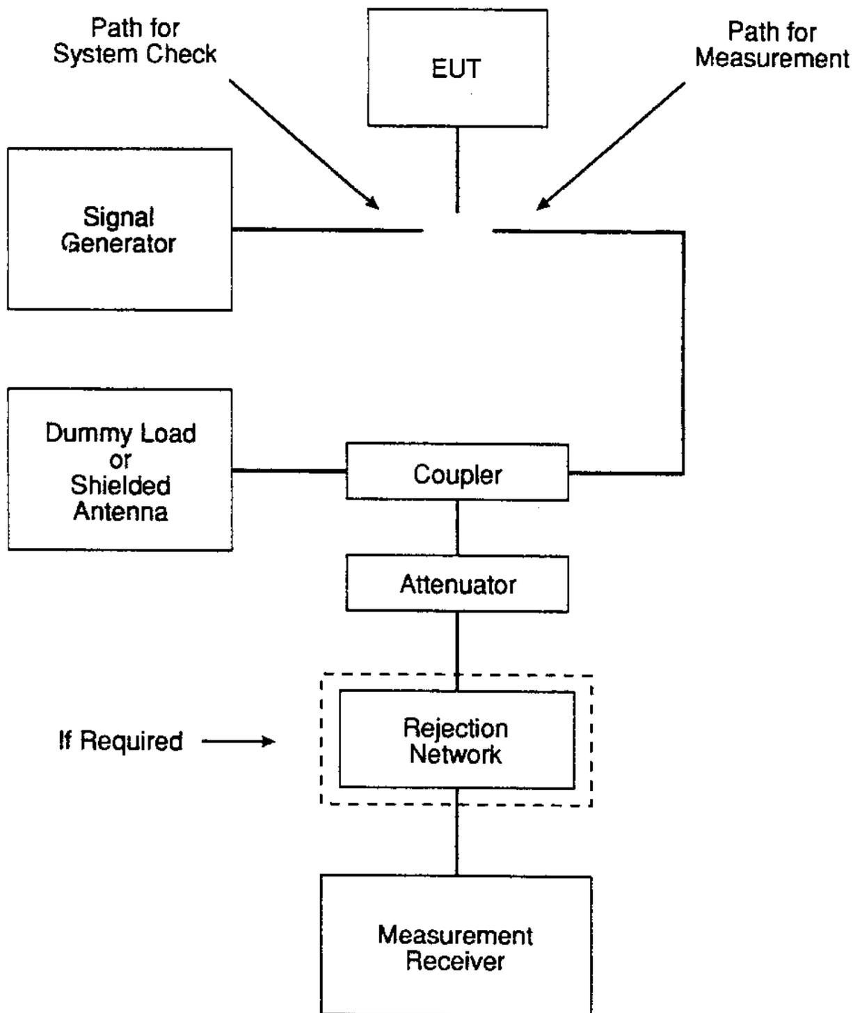
FIGURE CE106-2. Setup for high power transmitter.
