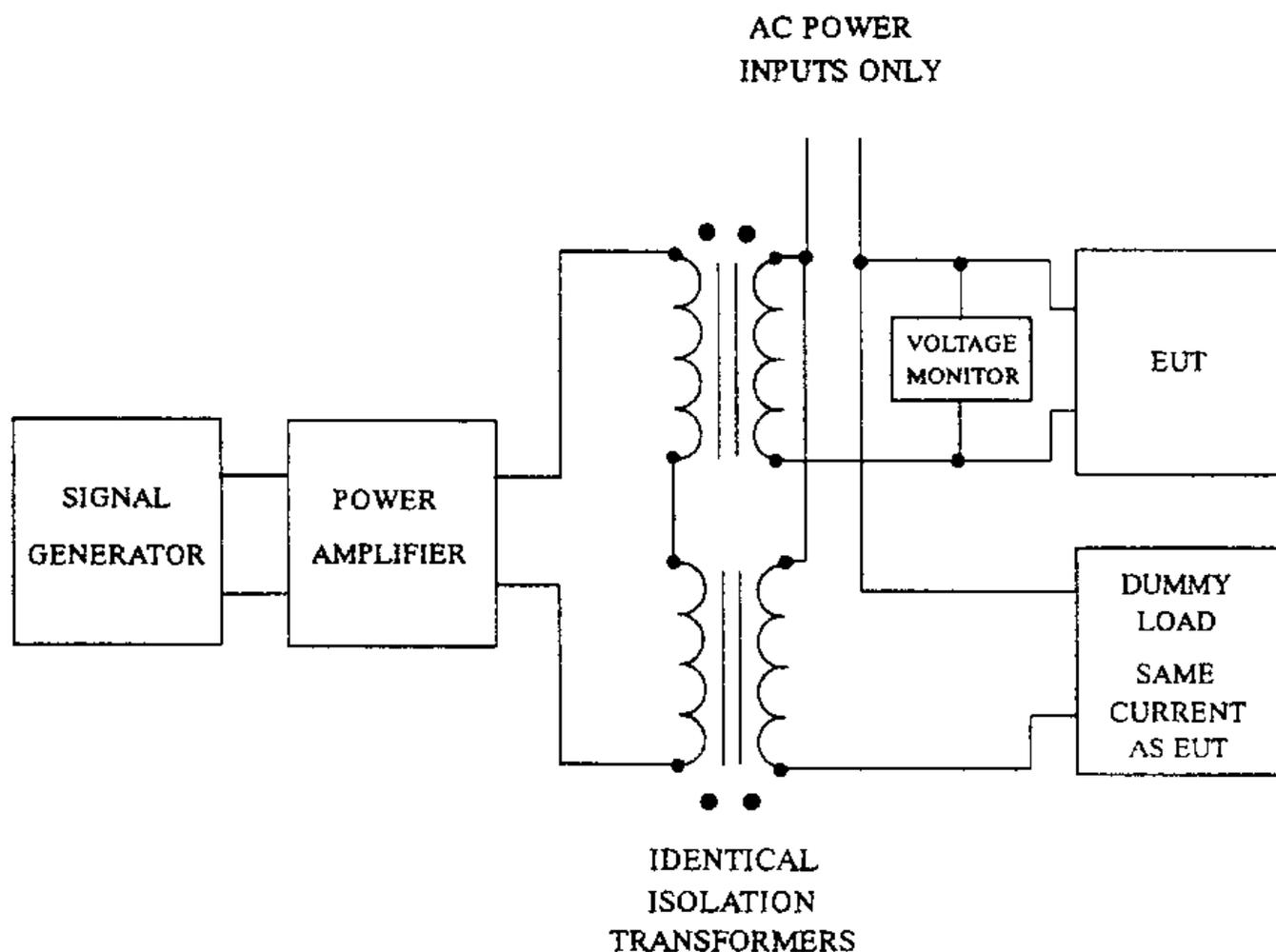
**FIGURE A-4. CS101 Power amplifier protection.**
