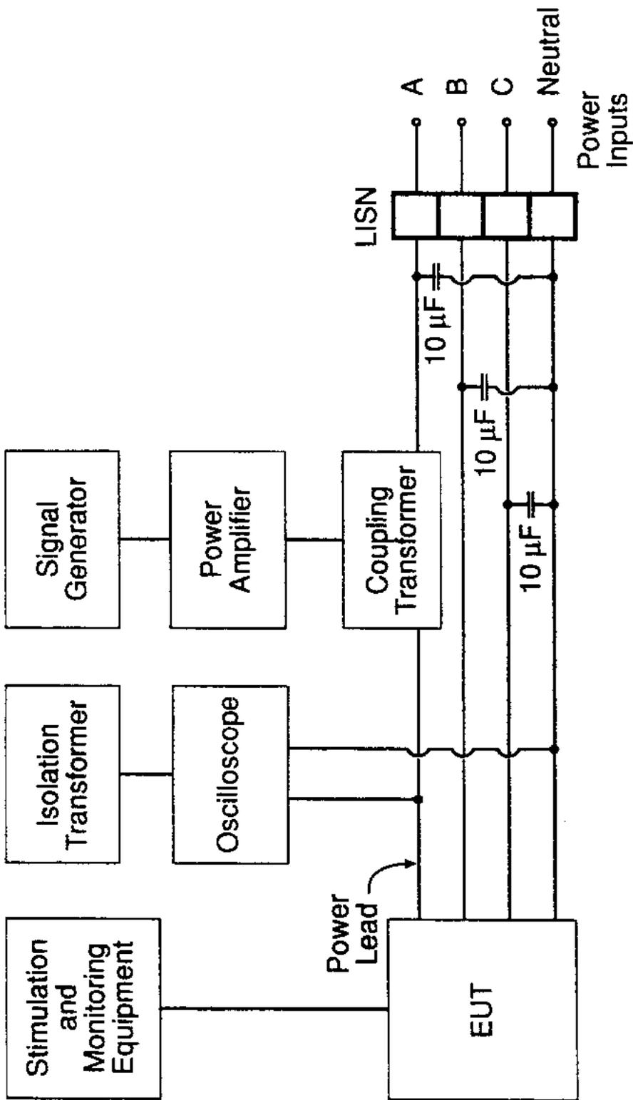
FIGURE CS101-4. Signal injection, 3-phase wye.
