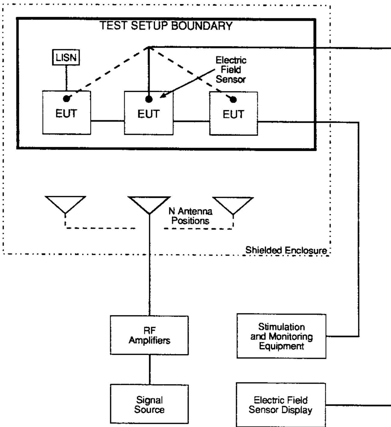
FIGURE RS103-2. Multiple test antenna locations for frequency > 200 MHz.
