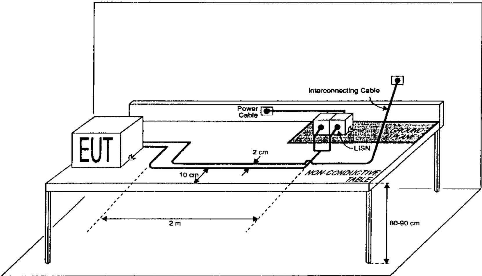
FIGURE 3. Test setup for non-conductive surface mounted EUT.
