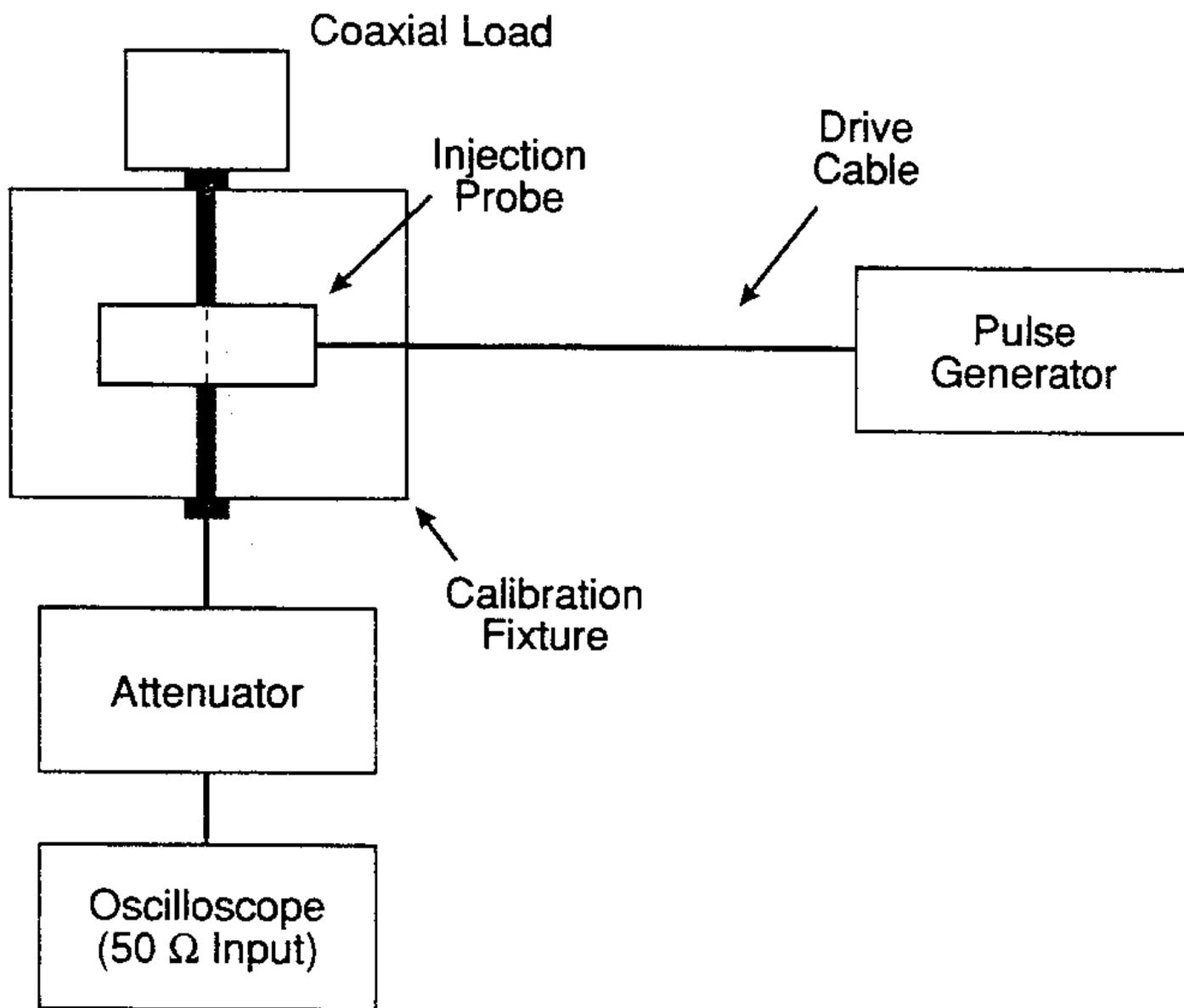
FIGURE CS115-1. Calibration setup.
