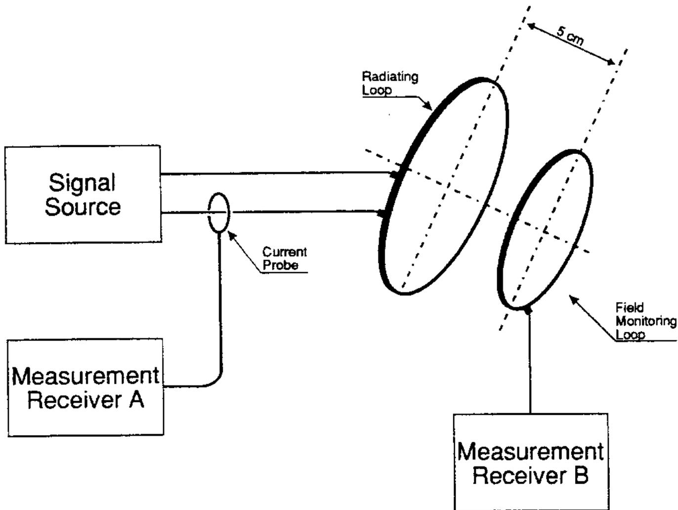
FIGURE RS101-2. Calibration of the radiating system.
