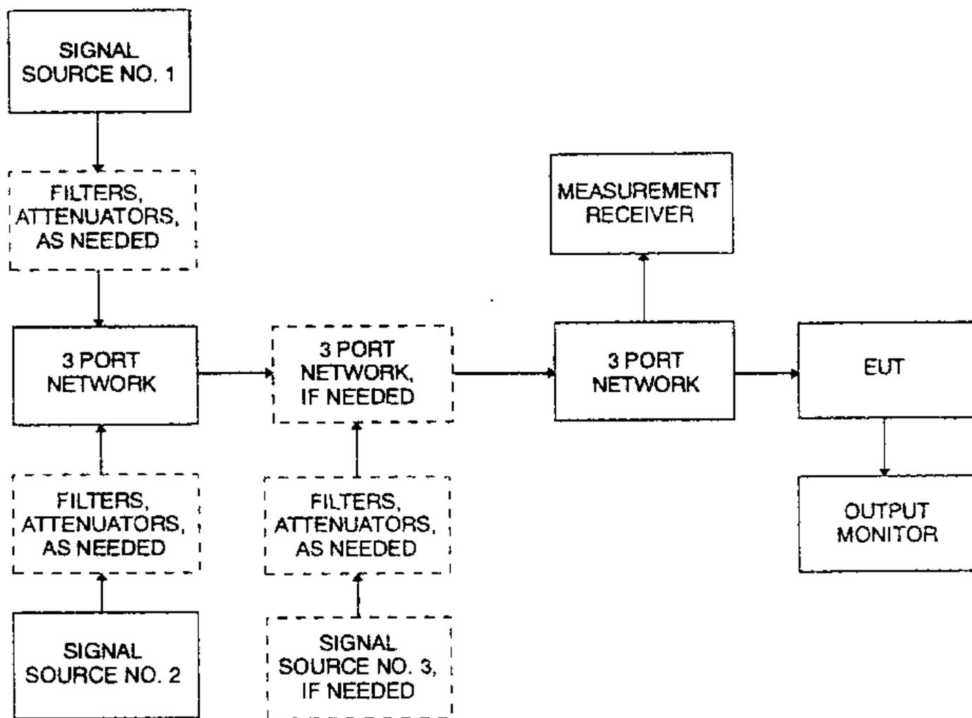
FIGURE A-5. CS103 General test setup.
