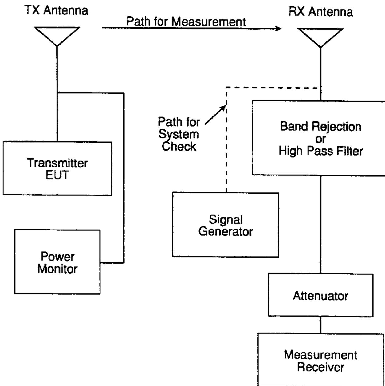
FIGURE RE103-1. Calibration and test setup for radiated harmonics and spurious emissions, 10 kHz to 1 GHz.
