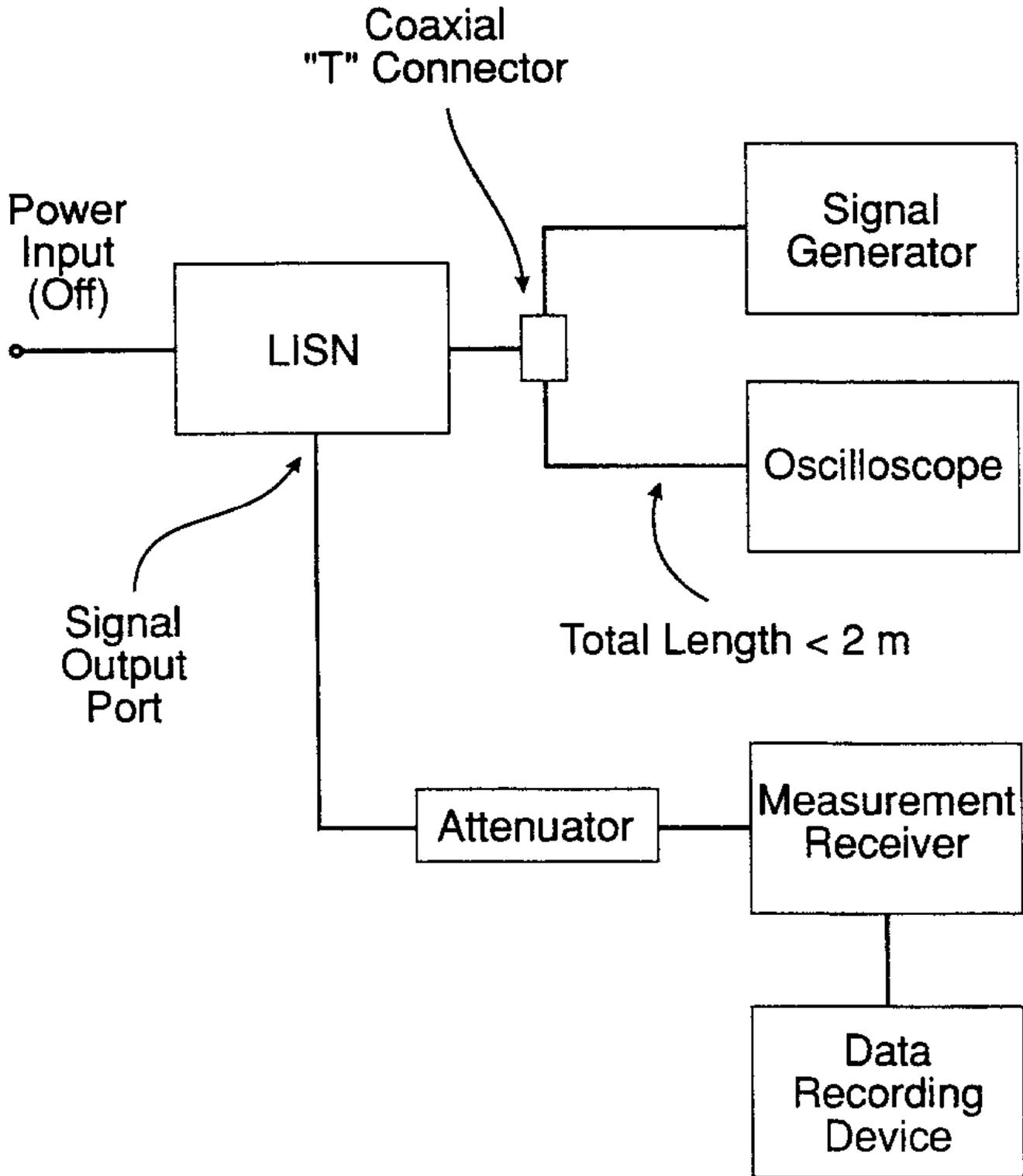
FIGURE CE102-1. Measurement system check setup.
