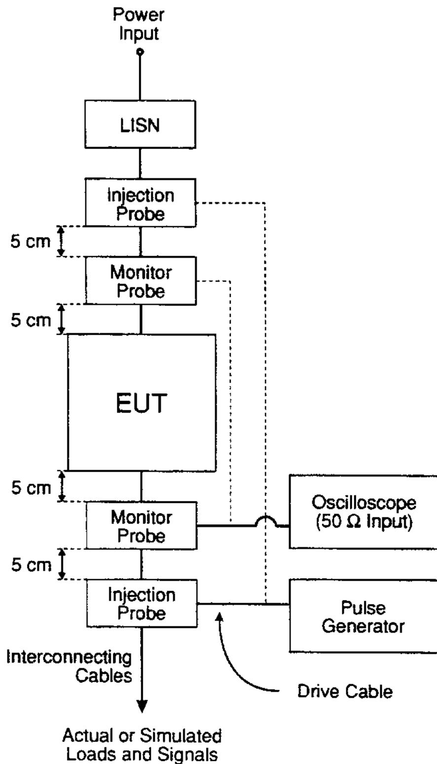
FIGURE CS115-2. Bulk cable injection.
