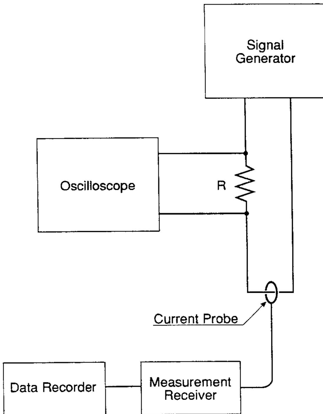
FIGURE CE101-1. Measurement system check setup.
