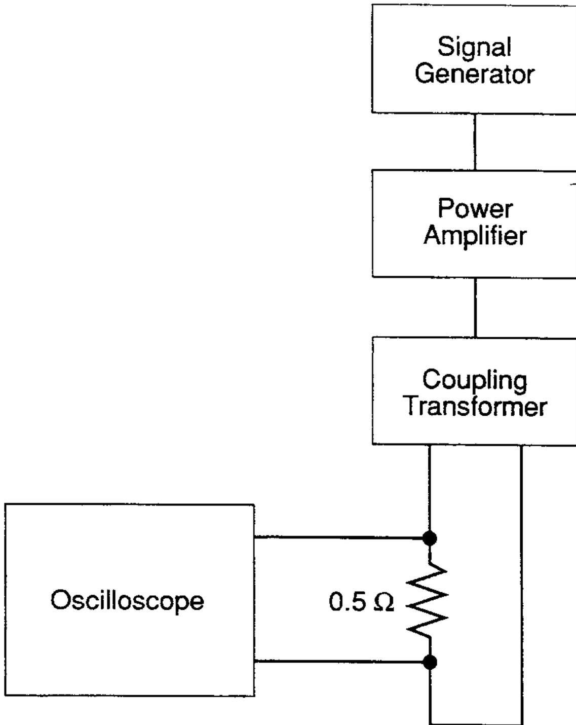
FIGURE CS101-1. Calibration.
