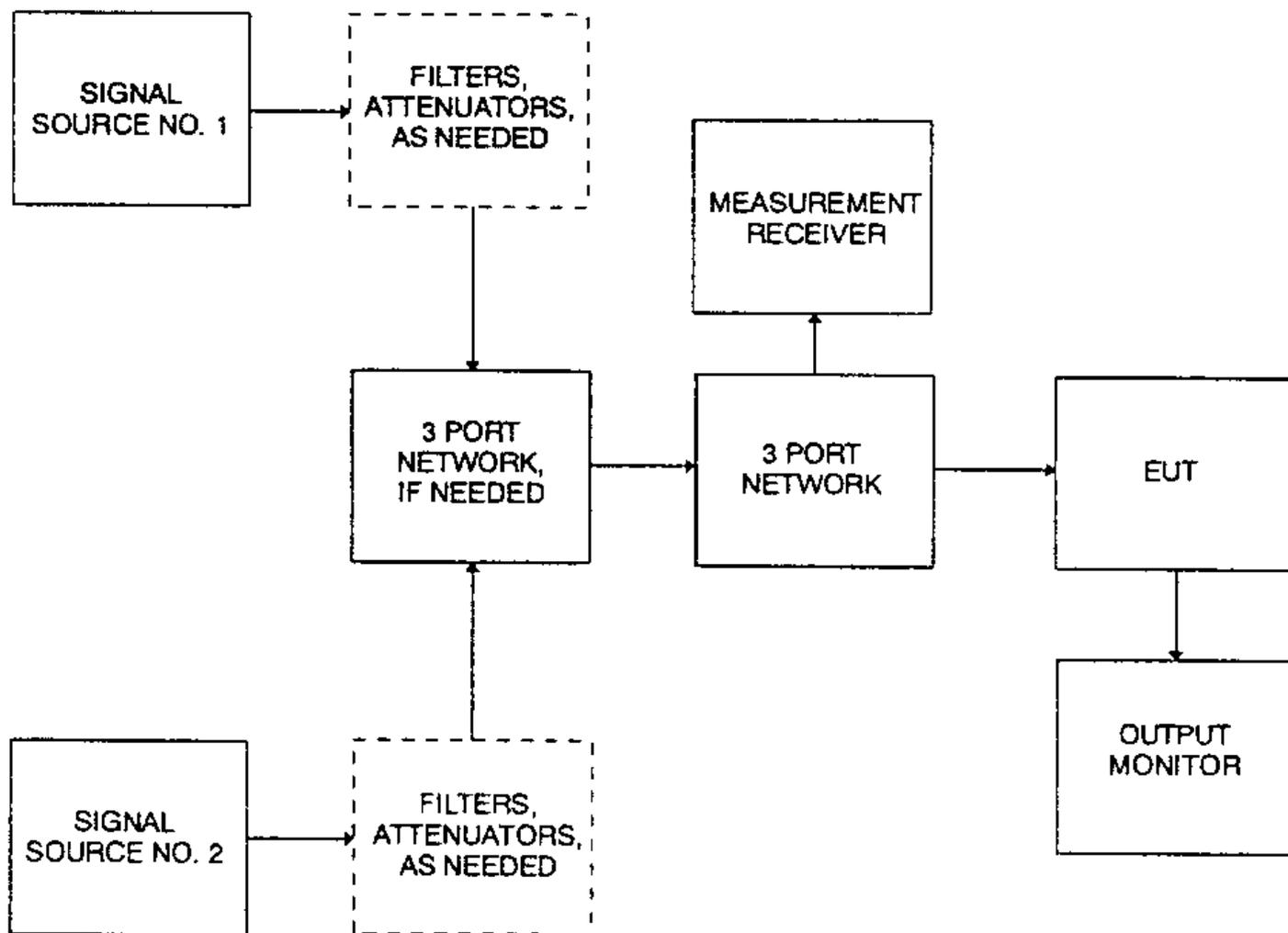
FIGURE A-7. CS105 General test setup.
