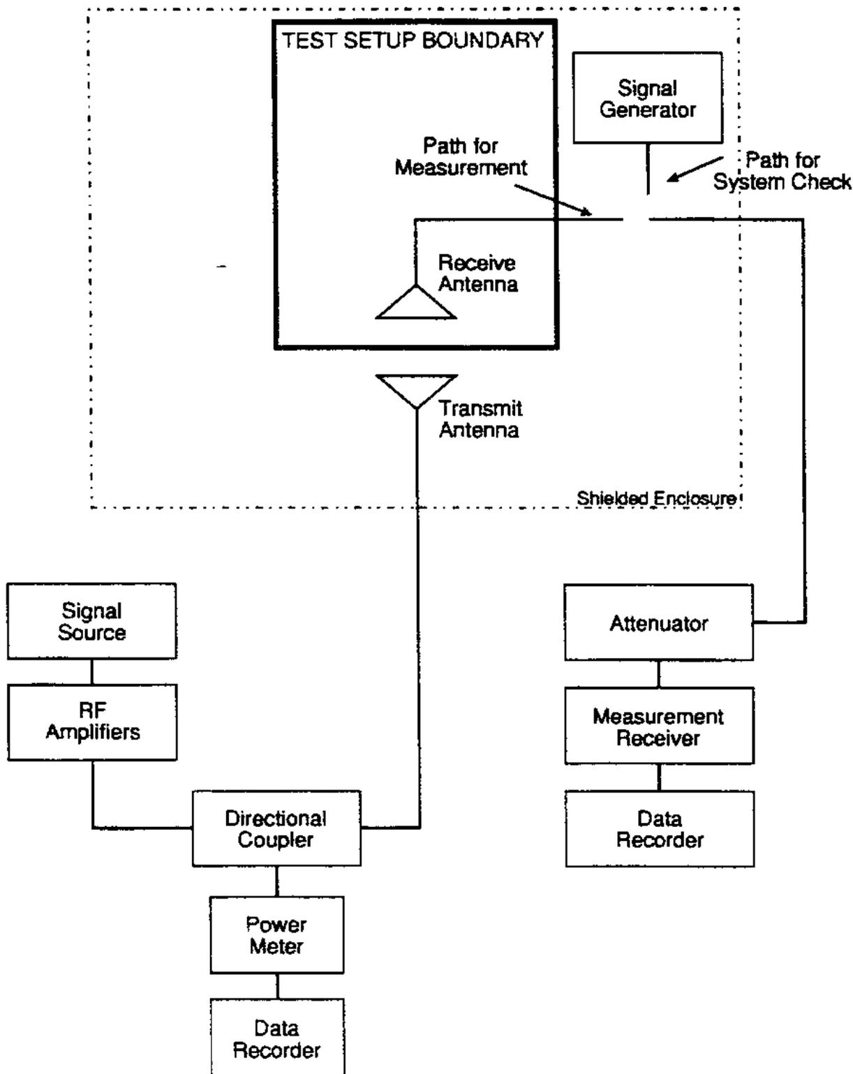
FIGURE RS103-4. Receive antenna method (1 to 40 GHz).
