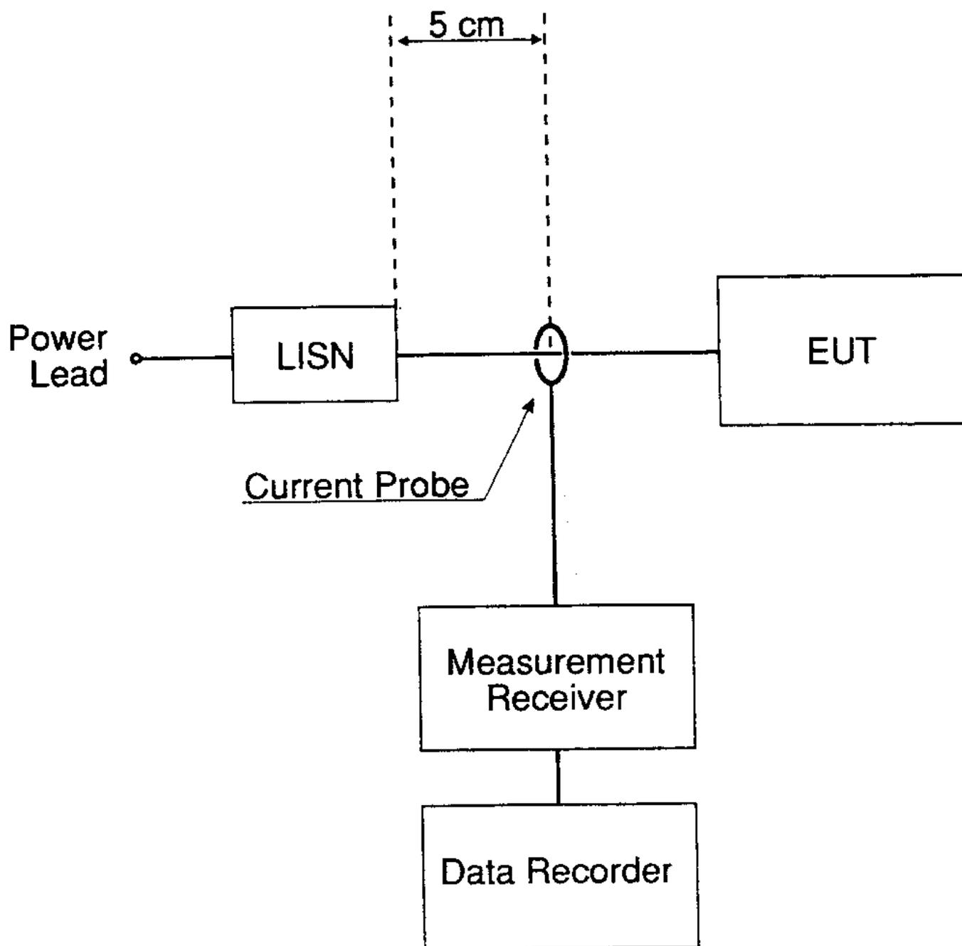
FIGURE CE101-2. Measurement setup.
