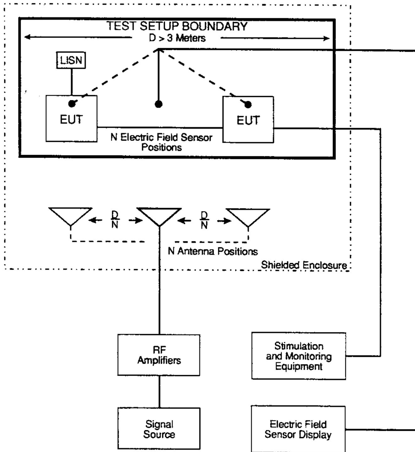
FIGURE RS103-3. Multiple test antenna locations for N positions,  $D > 3$  meters.
