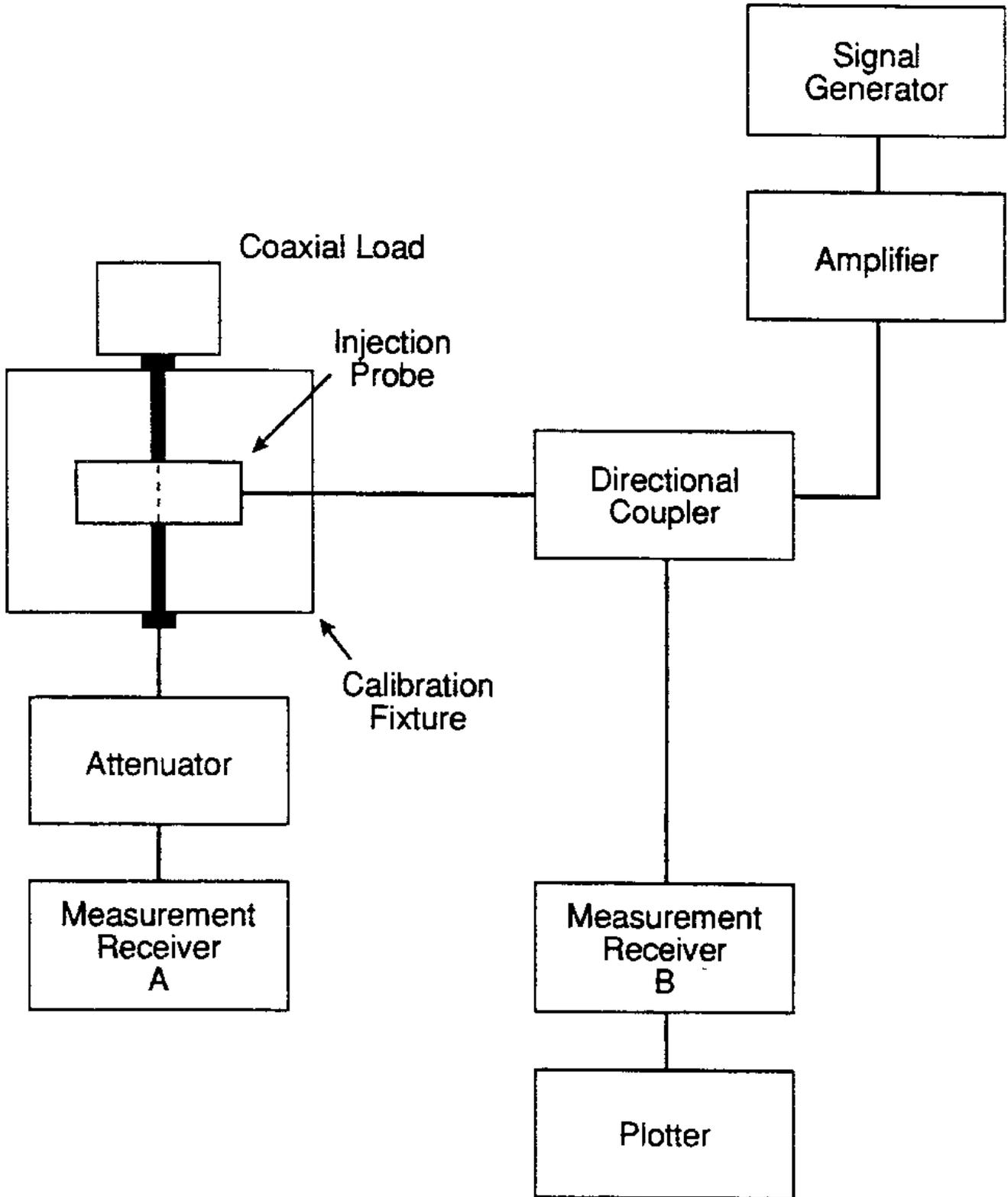
FIGURE CS114-1. Calibration setup.
