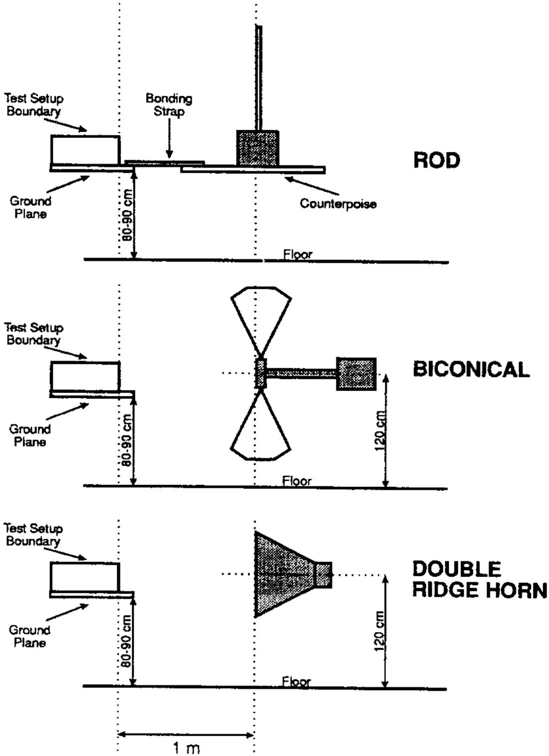
FIGURE RE102-2. Antenna positioning.
