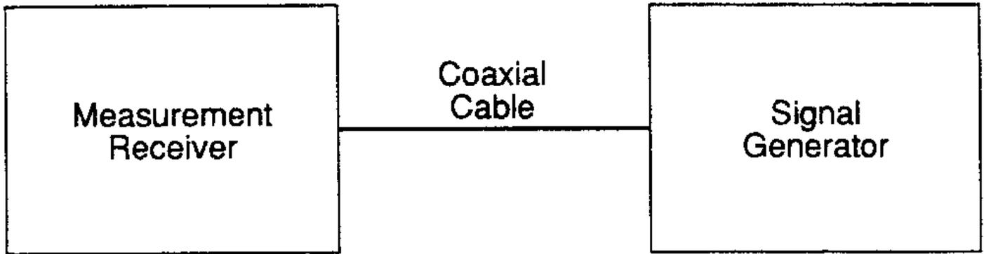
FIGURE RE101-2. Calibration configuration.
