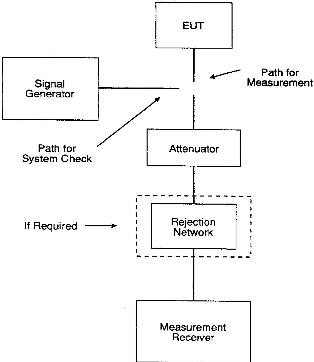
FIGURE CE106-1. Setup for low power transmitter.
