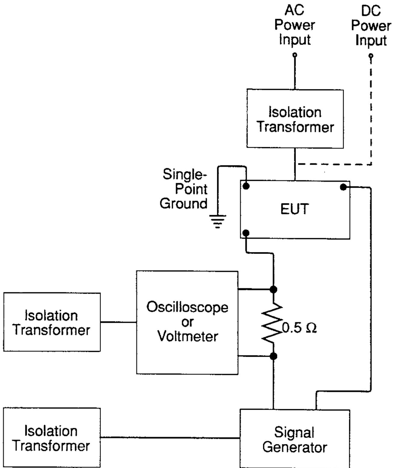
FIGURE CS109-1. Test Configuration.
