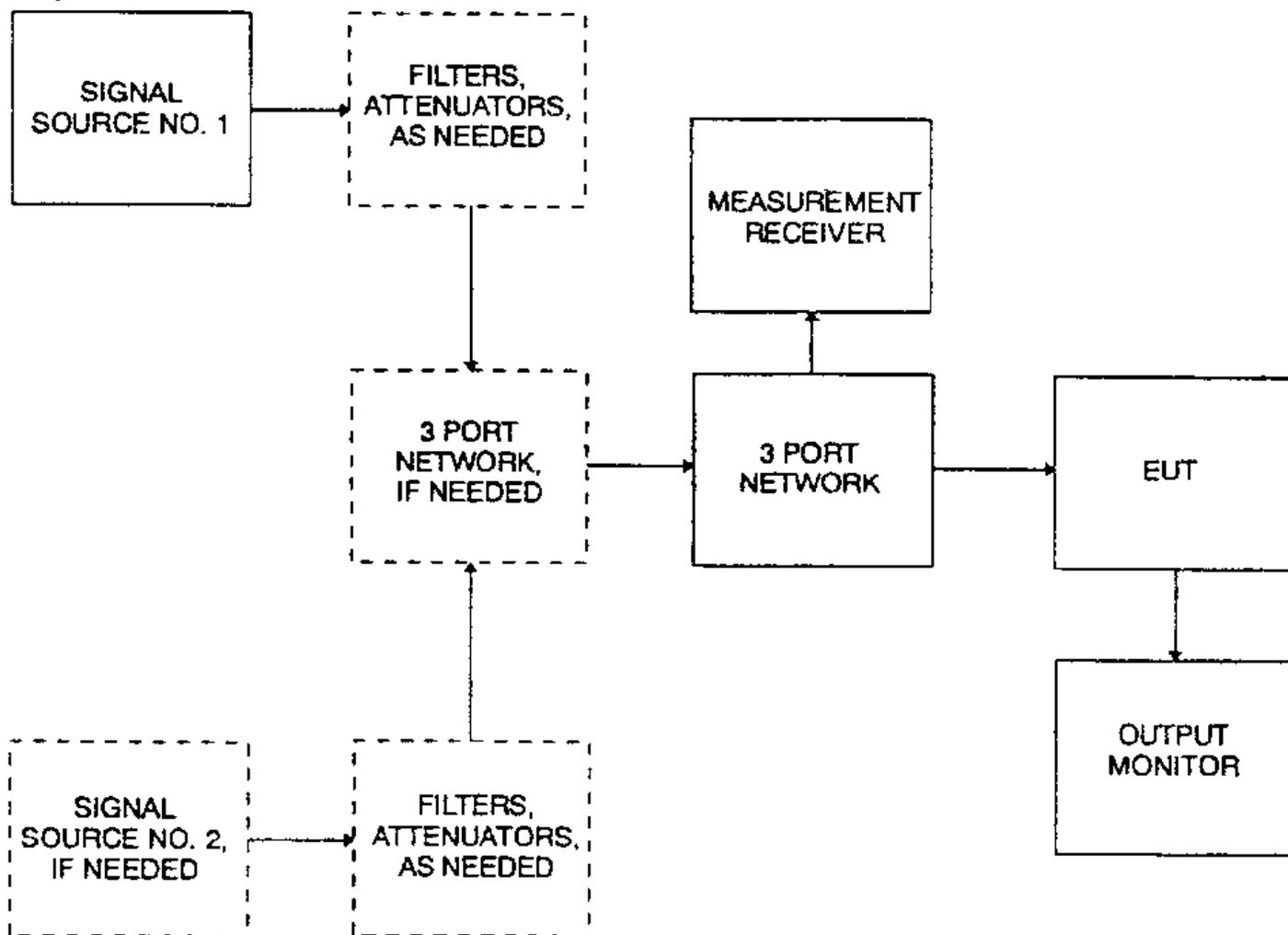
FIGURE A-6. CS104 General test setup.
