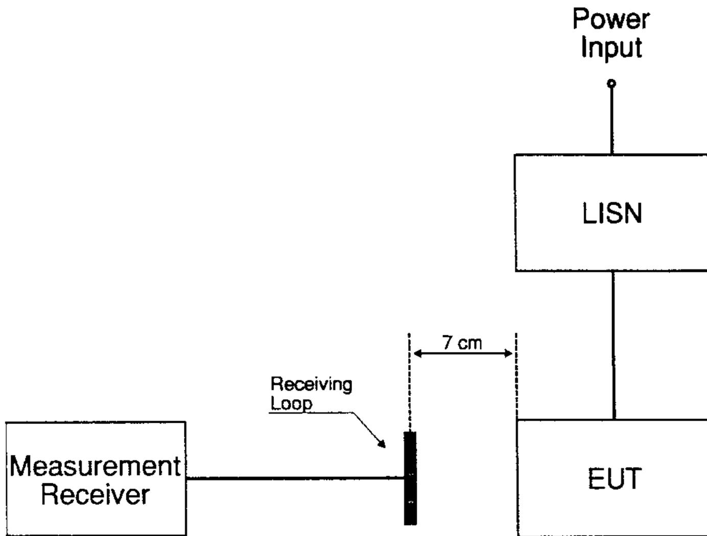
FIGURE RE101-3. Typical Test Setup for Radiated Emissions, Magnetic Field, 30 Hz to 100 kHz.
