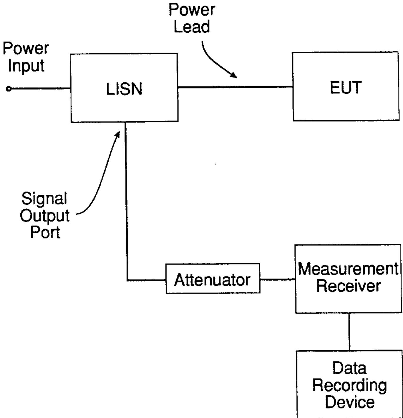
FIGURE CE102-2. Measurement setup.
