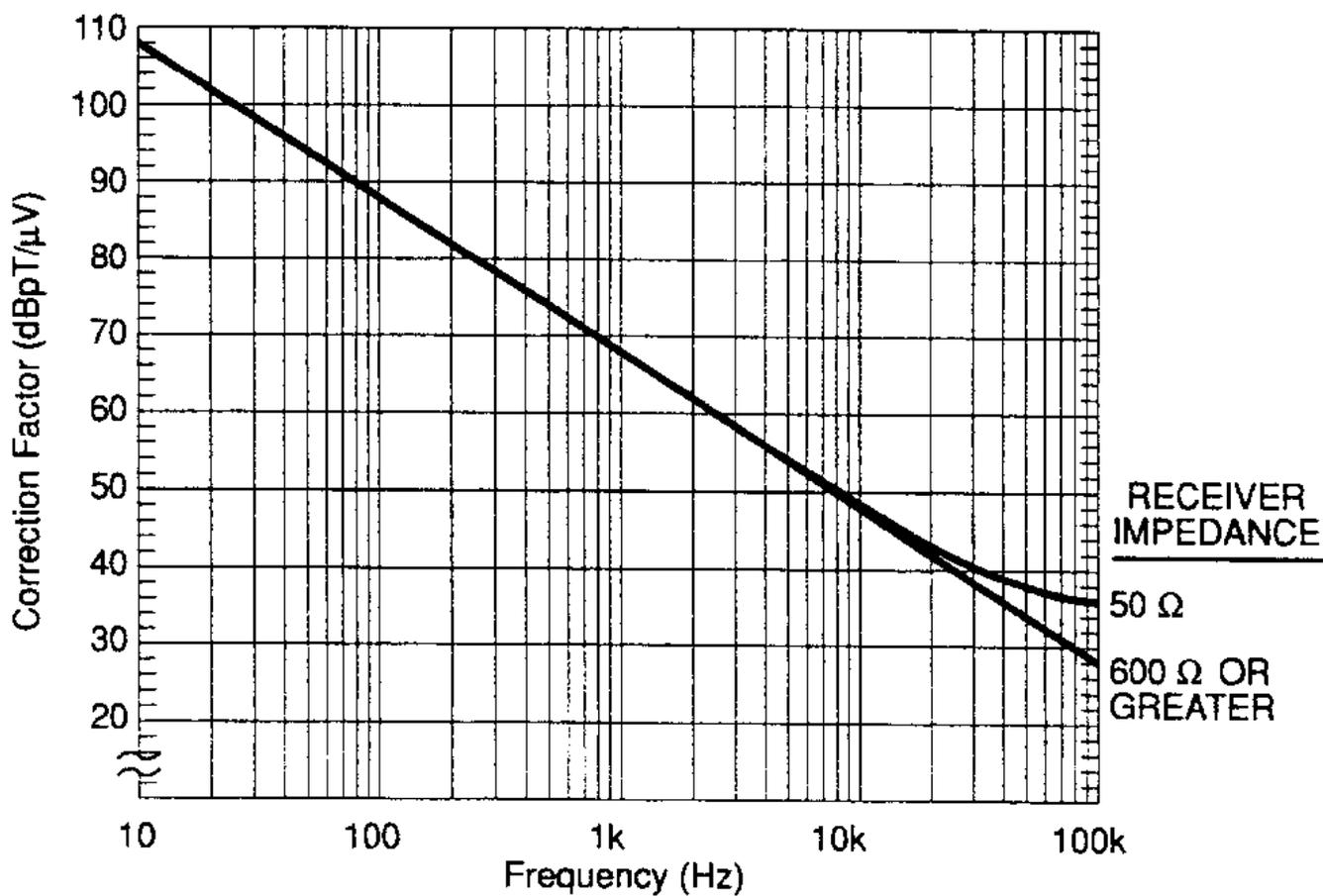
FIGURE RS101-1. Loop sensor correction factor.
