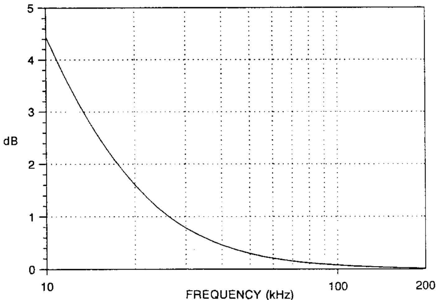
FIGURE A-3. Correction factor for LISN capacitor.
