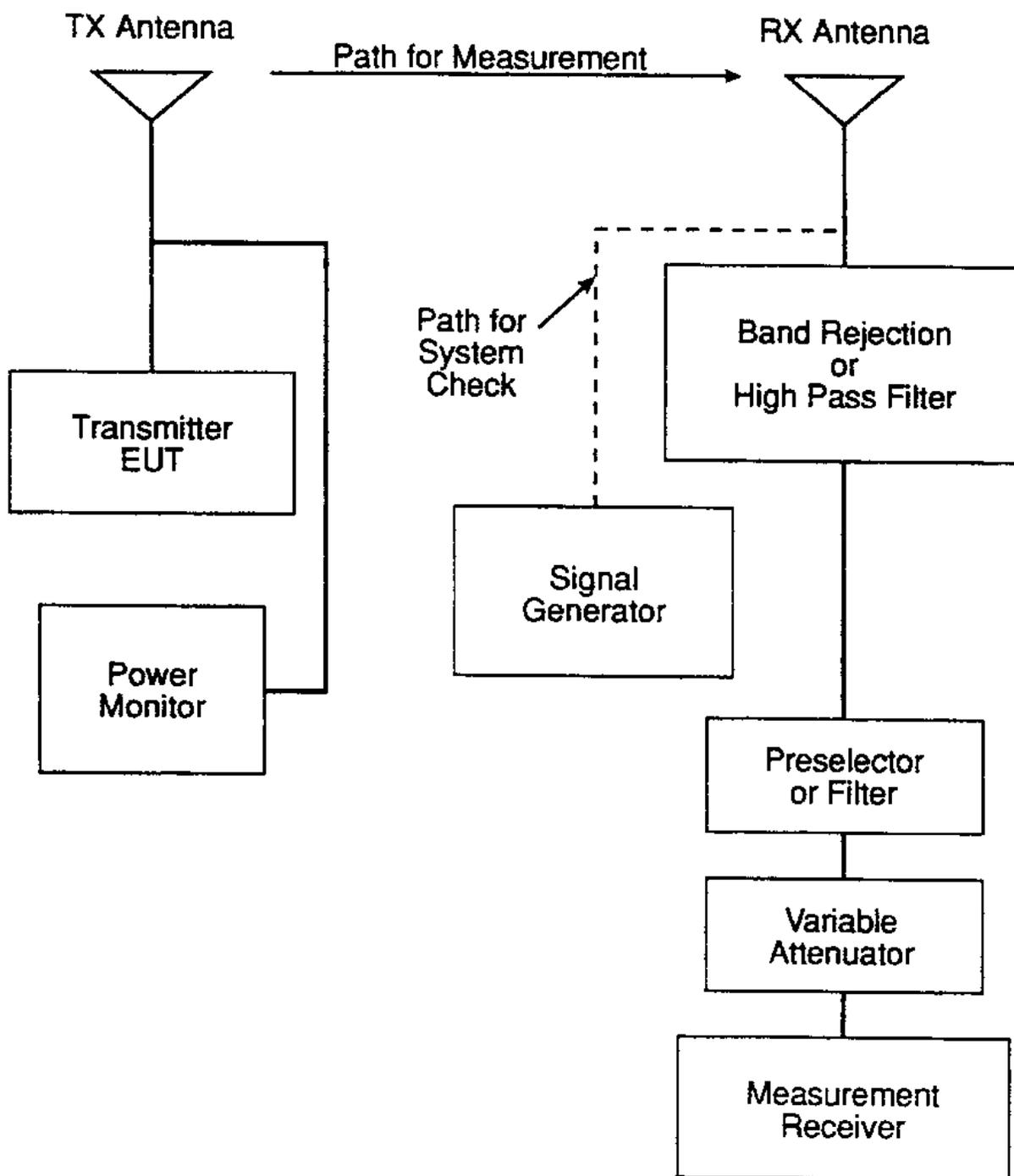
FIGURE RE103-2. Calibration and test setup for radiated harmonics and spurious emissions, 1 GHz to 40 GHz.
