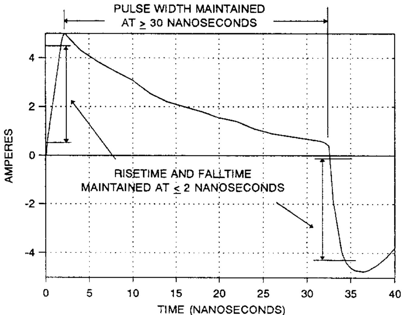
FIGURE A-11. Typical CS115 calibration fixture waveform.
