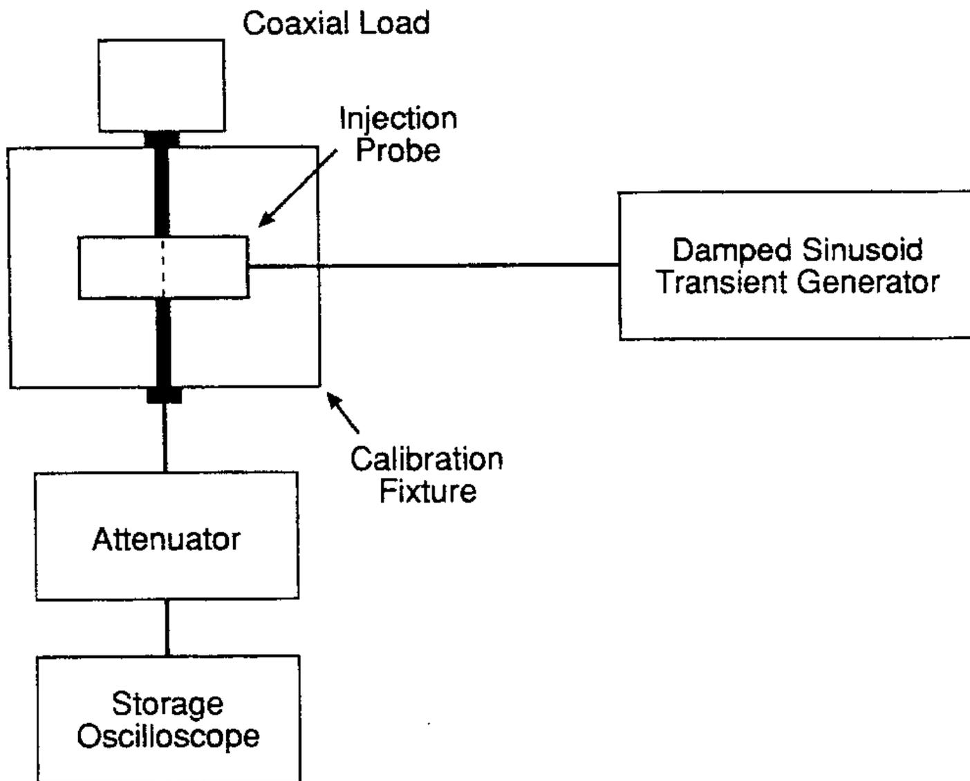
FIGURE CS116-1. Typical test setup for calibration of test waveform.
