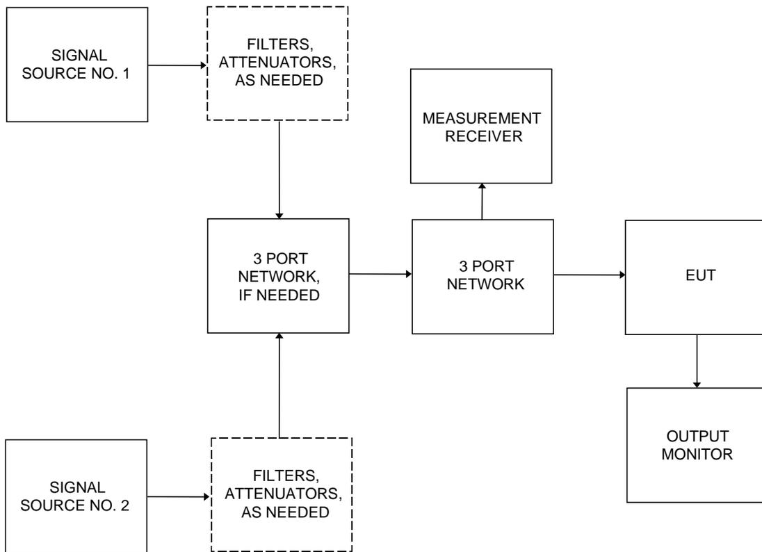
**FIGURE A-8. CS105 General test setup.**
