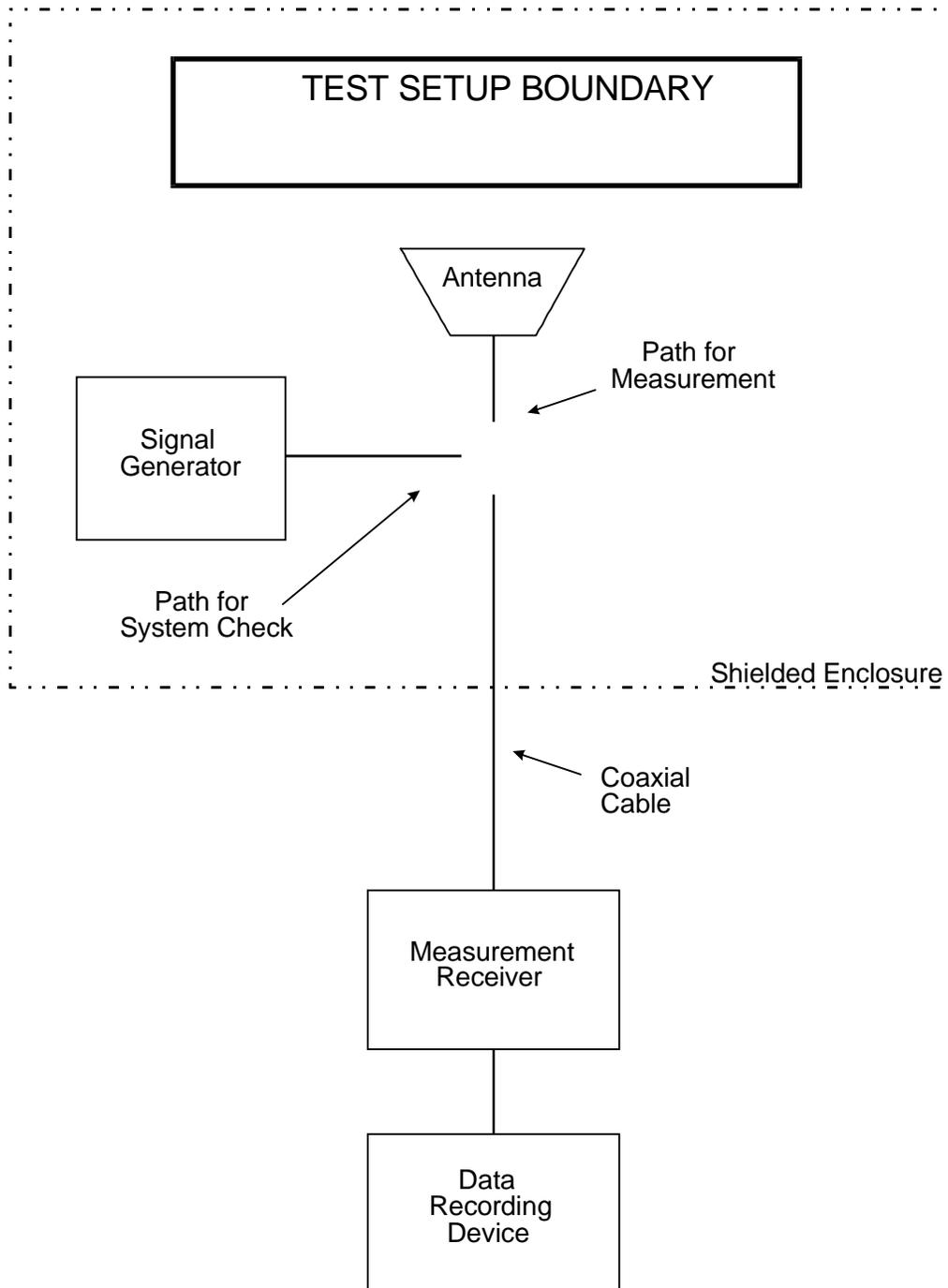
**FIGURE RE102-5. Basic test setup.**
