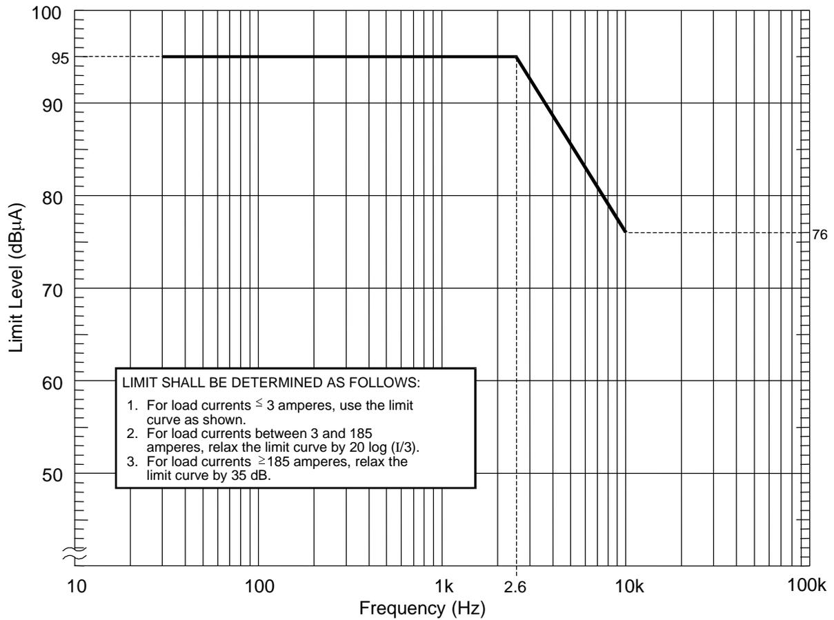
**FIGURE CE101-1. CE101 limit for submarine applications, DC.**
