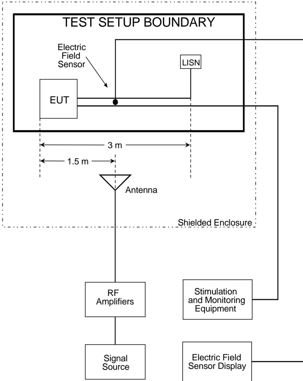
**FIGURE RS103-1. Test equipment configuration.**
