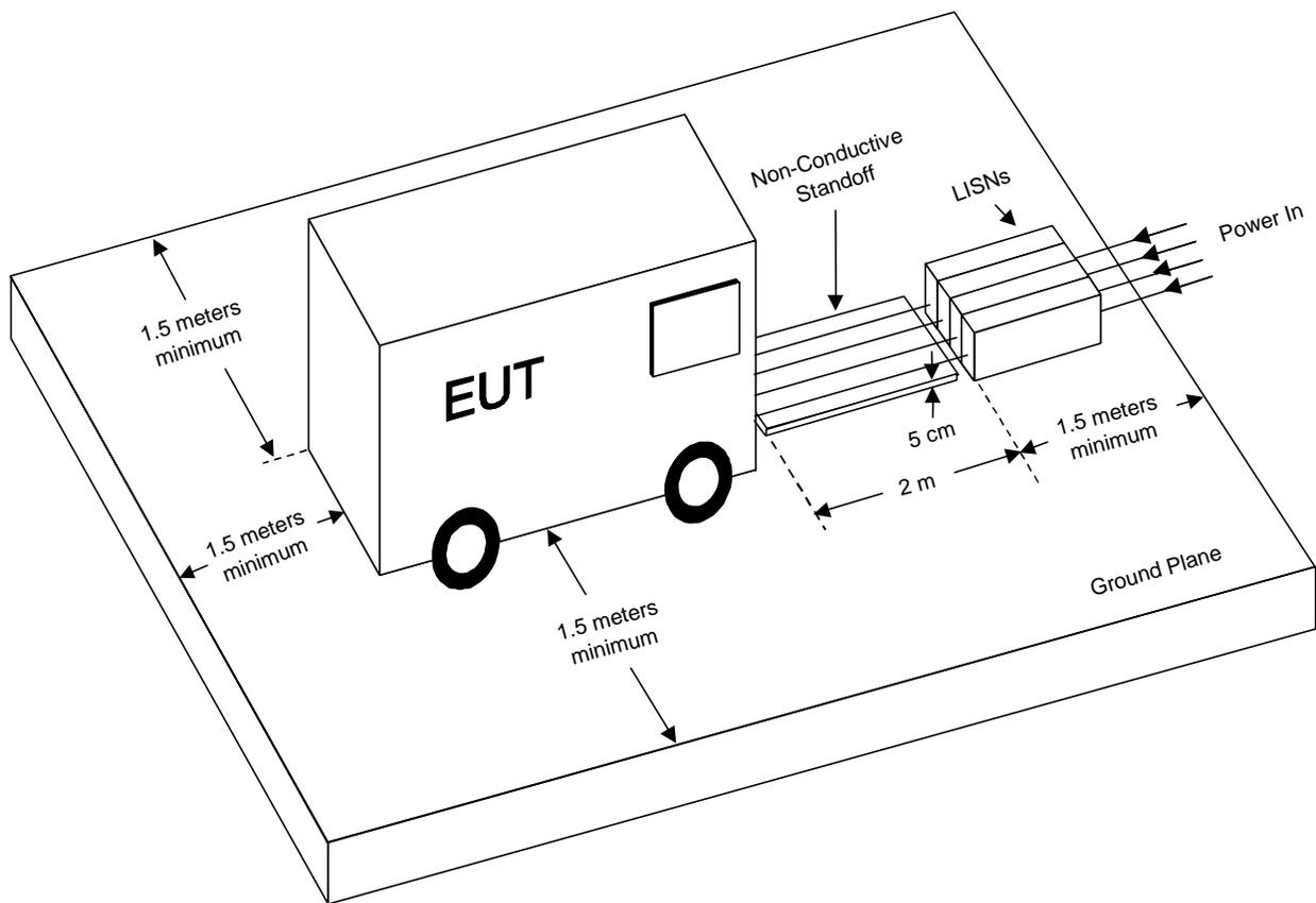
**FIGURE 5. Test setup for free standing EUT.**
