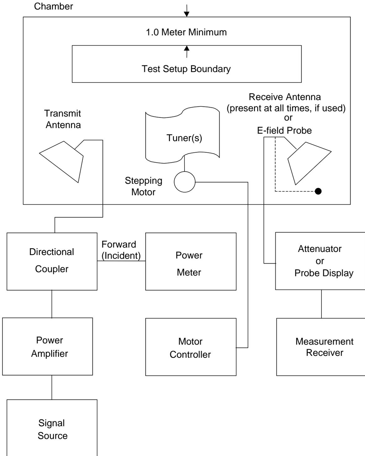
**FIGURE RS103-5. Reverberation chamber setup.**
