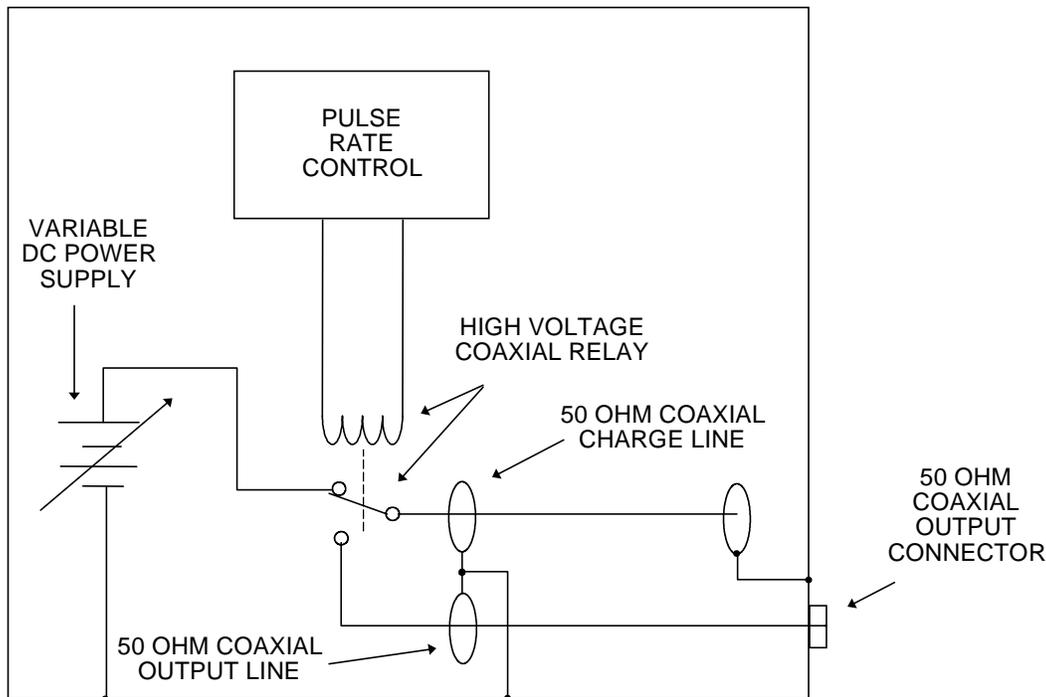
**FIGURE A-12. Circuit diagram of CS115 pulse generator.**
