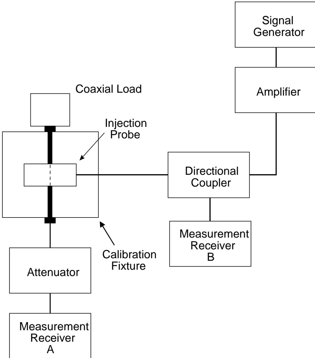
**FIGURE CS114-3. Calibration setup.**
