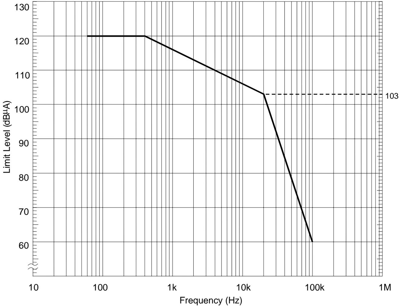
**FIGURE CS109-1. CS109 limit for all applications**
