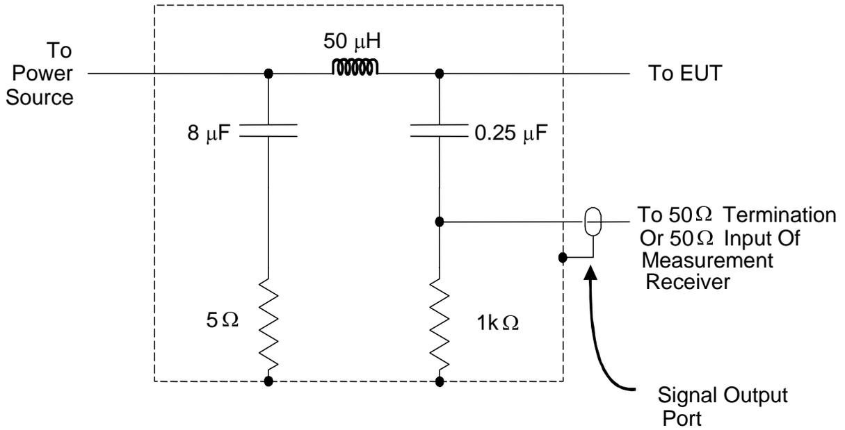
**FIGURE 6. LISN schematic.**
