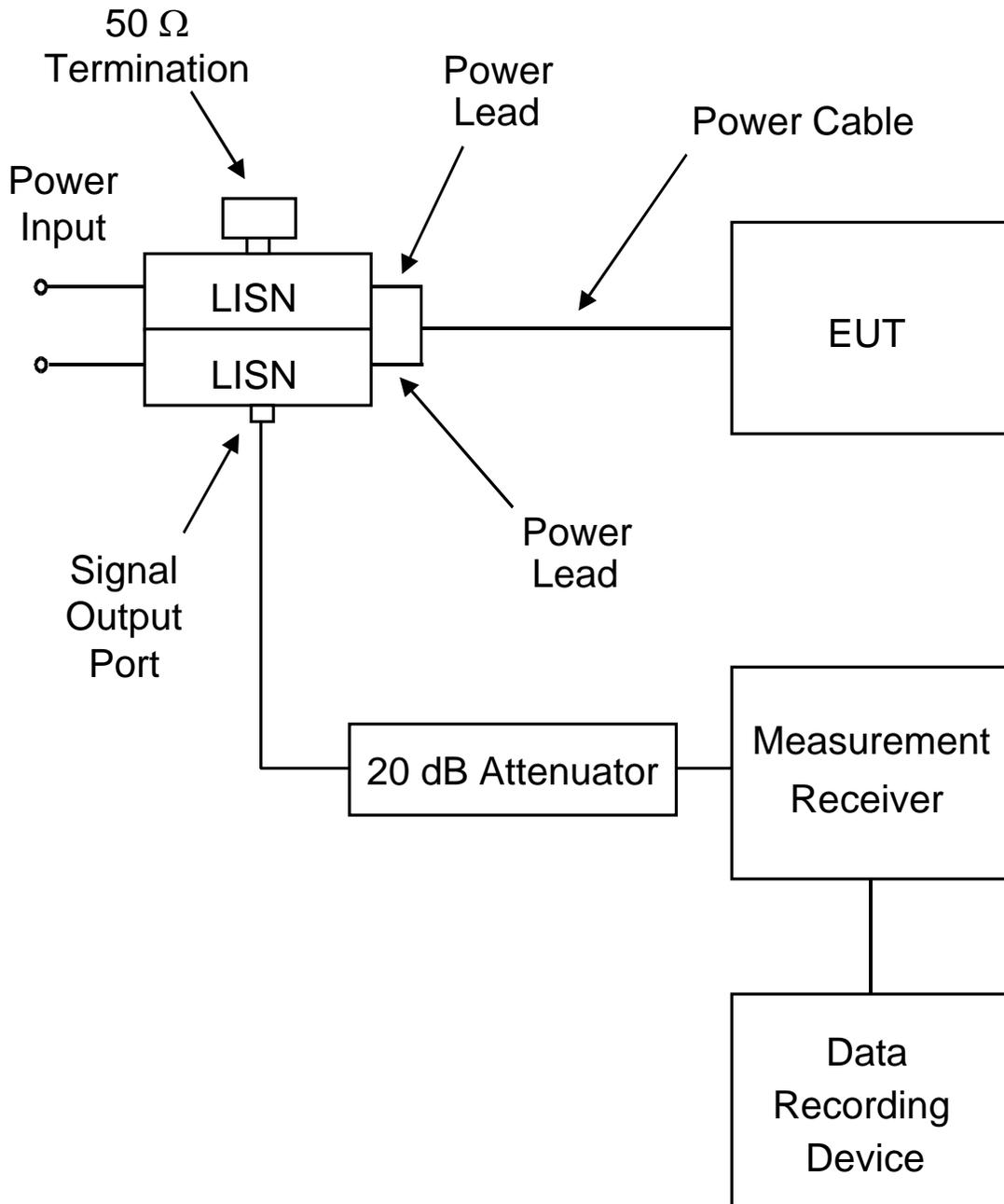
**FIGURE CE102-3. Measurement setup.**
