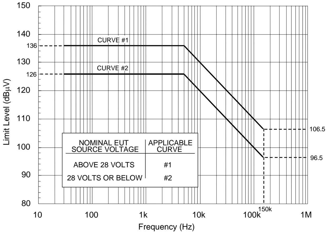
**FIGURE CS101-1. CS101 voltage limit for all applications.**
