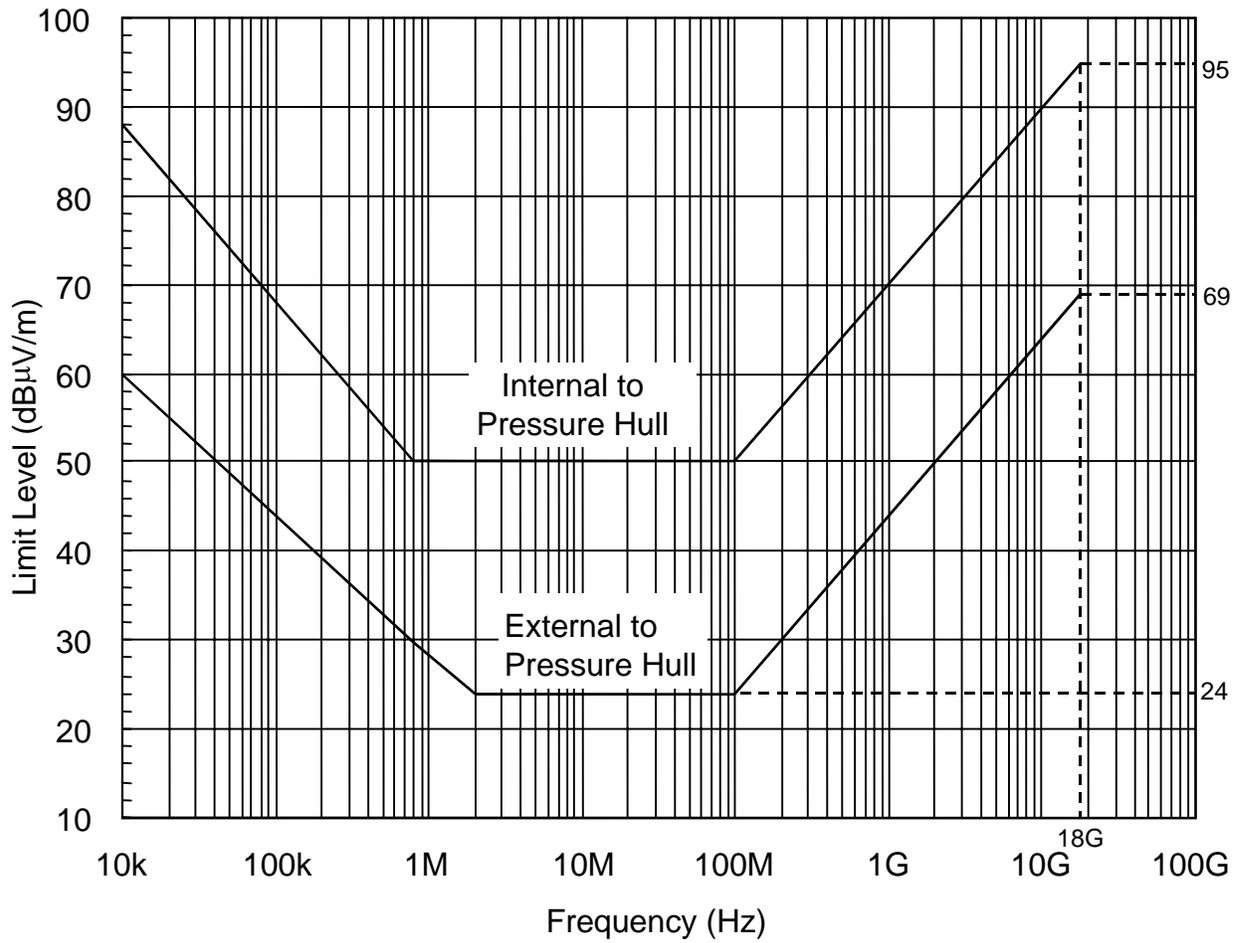
**FIGURE RE102-2. RE102 limit for submarine applications.**
