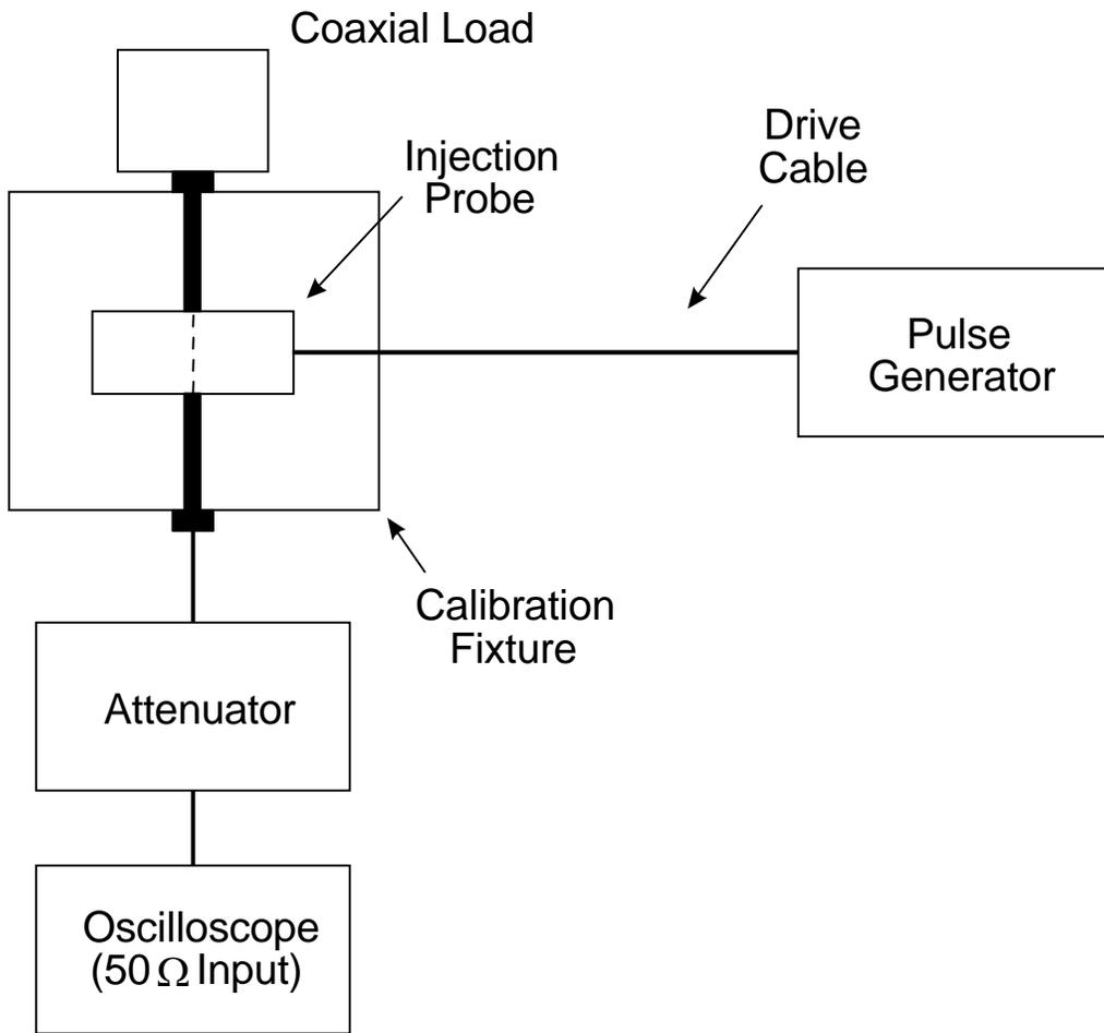
**FIGURE CS115-2. Calibration setup.**
