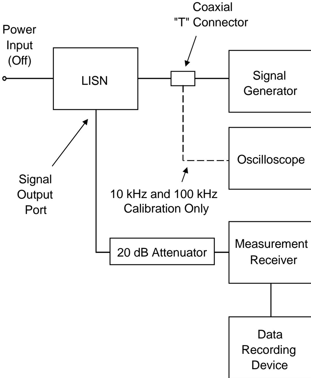
**FIGURE CE102-2. Measurement system check setup.**
