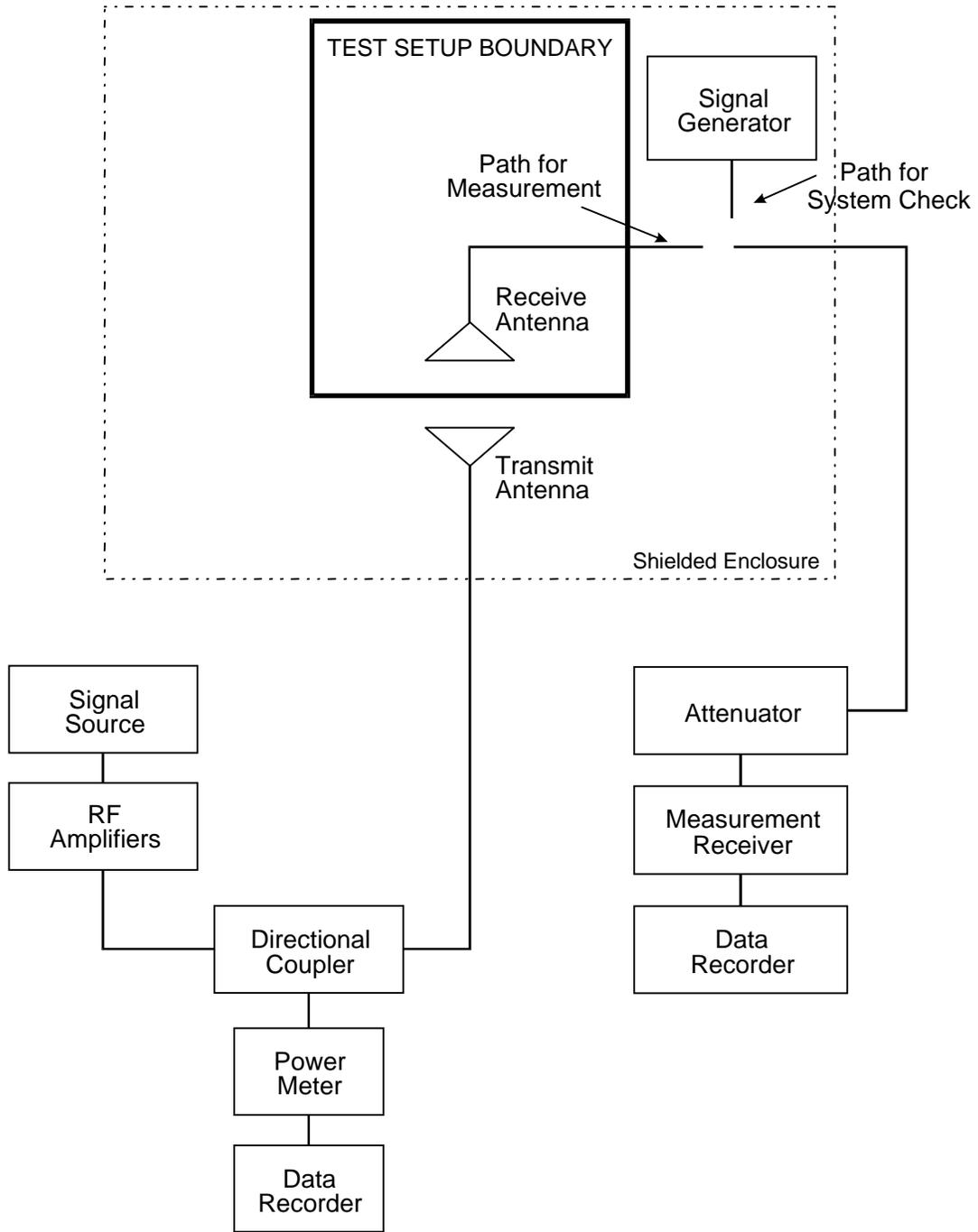
**FIGURE RS103-4. Receive antenna procedure (1 to 40 GHz).**
