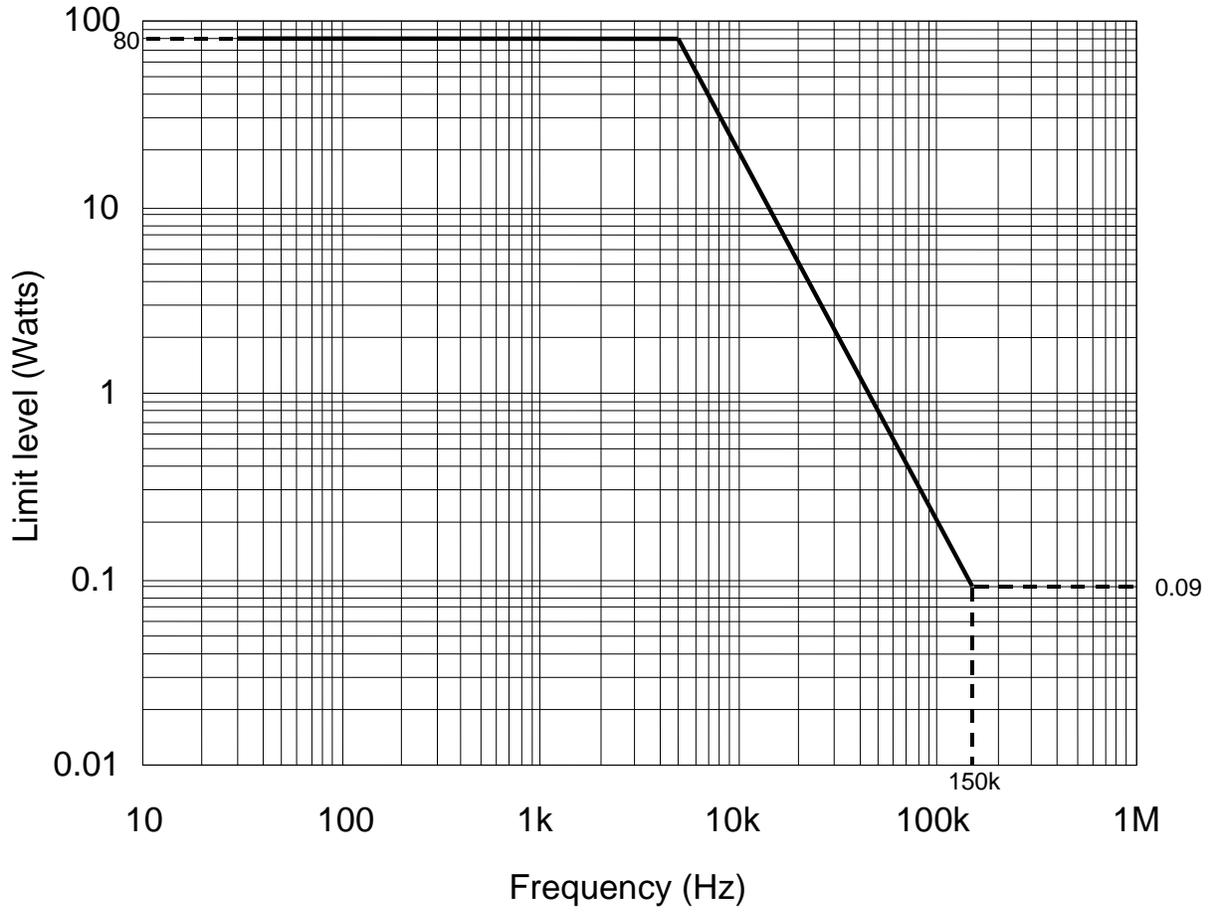
**FIGURE CS101-2. CS101 power limit for all applications.**
