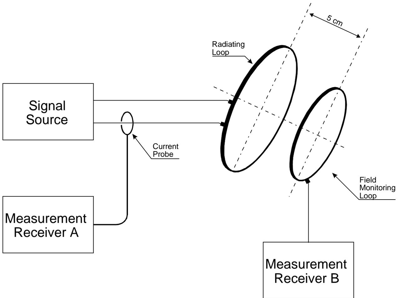
**FIGURE RS101-3. Calibration of the radiating system.**
