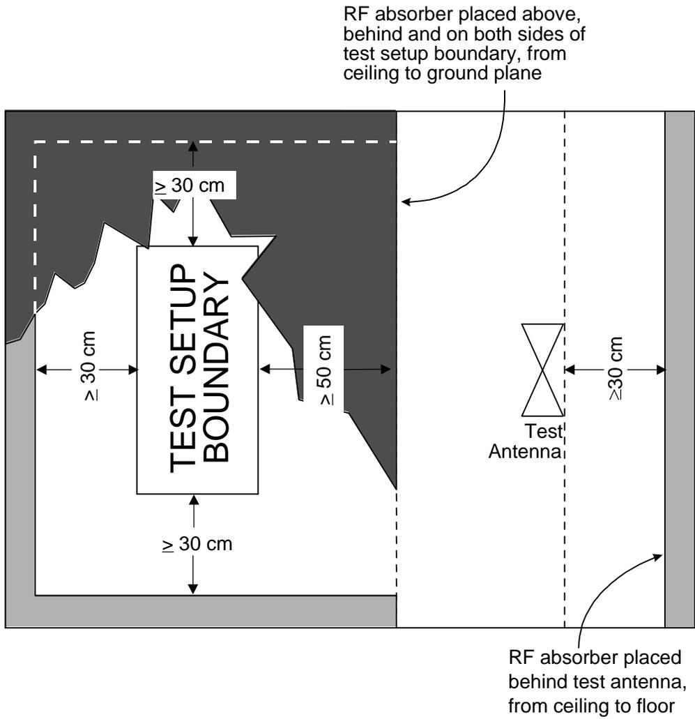
**FIGURE 1. RF absorber loading diagram.**
