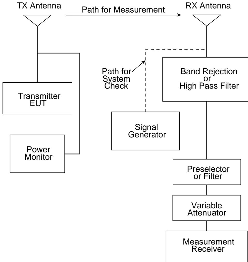
**FIGURE RE103-2. Calibration and test setup for radiated harmonics and spurious emissions, 1 GHz to 40 GHz.**
