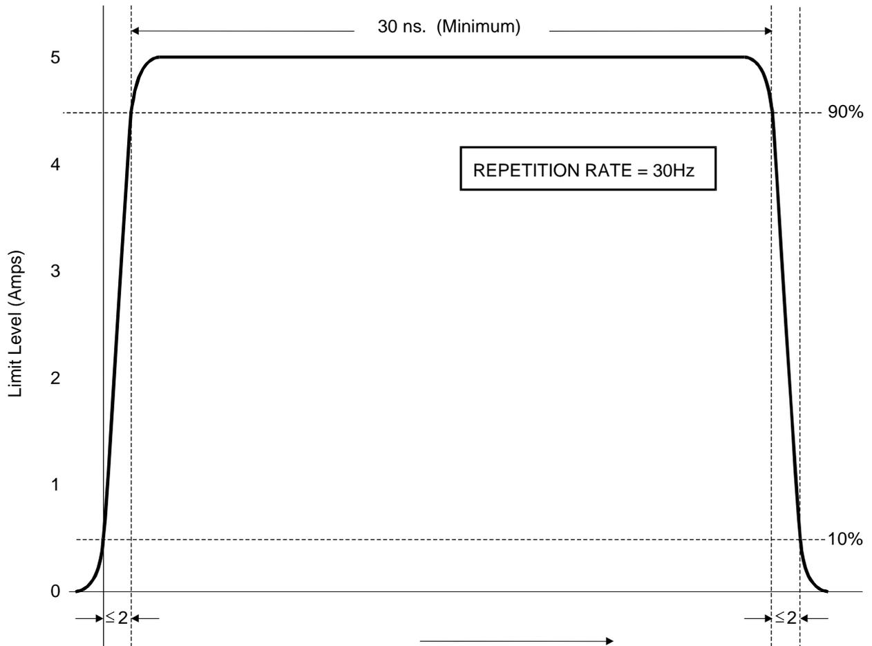
**FIGURE CS115-1. CS115 signal characteristics for all applications.**
