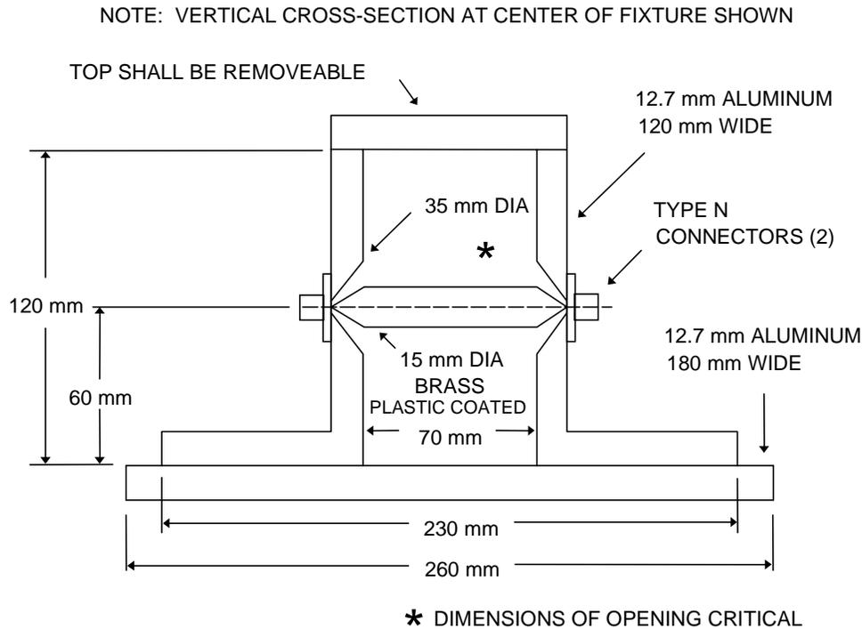
**FIGURE A-9. Typical CS114 calibration fixture.**
