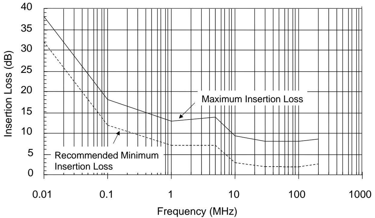
**FIGURE CS114-2. Maximum insertion loss for injection probes.**
