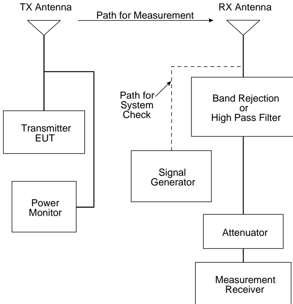
**FIGURE RE103-1. Calibration and test setup for radiated harmonics and spurious emissions, 10 kHz to 1 GHz.**
