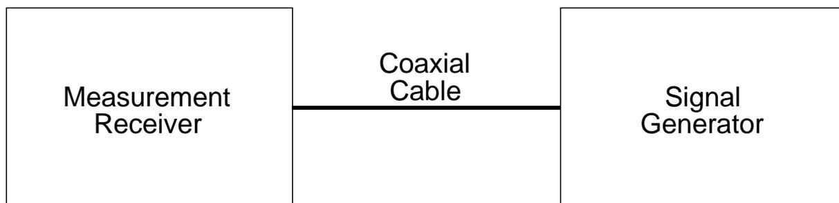
**FIGURE RE101-3. Calibration configuration.**
