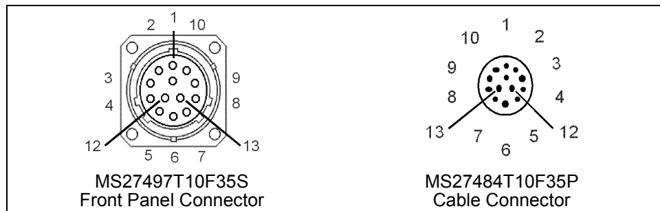
Figure 3-11. NTSC/Audio Connector Face
